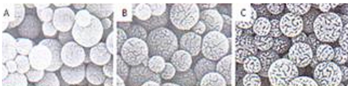
Figure 11. Porous spherical carbon particles for supercapacitor electrodes. Representative electron micrographs showing (A) Pristine carbon nanospheres prepared by HTS; (B) Carbon spheres after carbonization; (C) Carbon spheres after graphitization.
