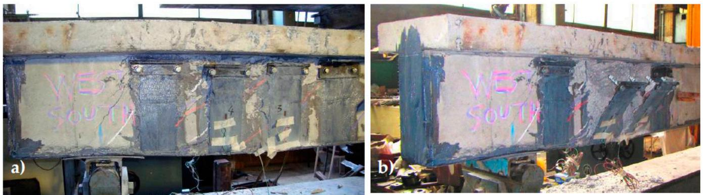
**Figure 23.** (a) The 3rd strengthening scheme (West part). (b) The widening of the shear diagonal cracks and the partial crushing of the concrete volume in the anchoring region reduced considerably the effectiveness of this anchoring scheme.
