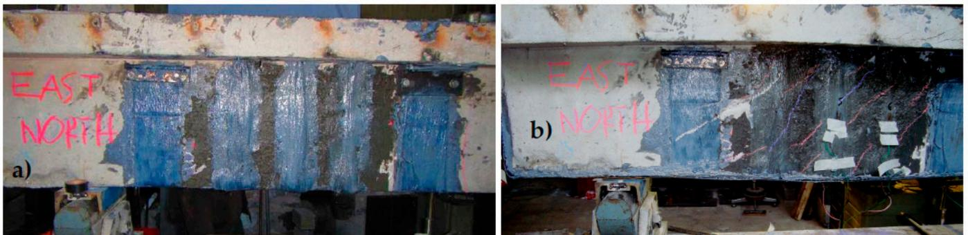
**Figure 19.** (a) The *2nd strengthening scheme* (East part). (b) Diagonal shear cracks at the East part of the prototype RC T-beam, which were checked by the applied CFRP anchor poles.
