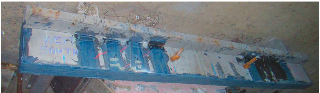
**Figure 21.** The 3rd strengthening scheme. Open hoop CFRP strips with mechanical anchors at the West part and closed hoop anchor ropes at the East part (The same as in Strengthening scheme 2). The flexural upgrade of the 3rd strengthening scheme consisted of five (5) CFRP layers (each 0.131 mm thick and 120 mm wide) attached at the bottom side of the T-beam specimen.
