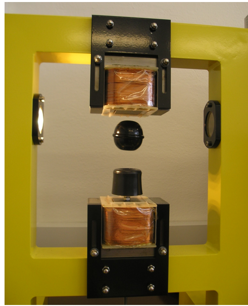
Figure 1. Laboratory Magnetic Levitation Plant from INTECO [25] having 2 electromagnets (coils). A levitating sphere ball should be positioned in the air-space.
