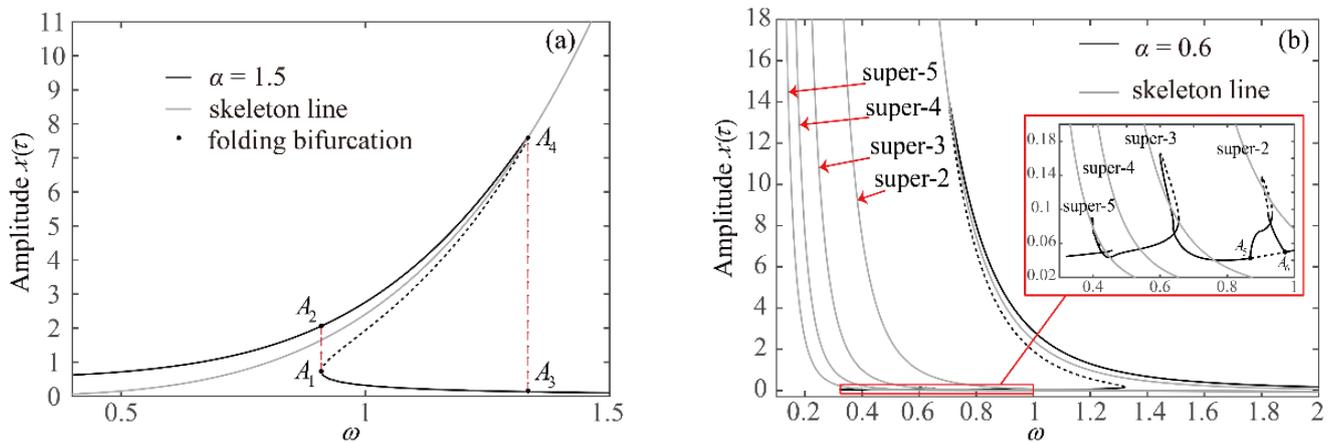
Figure 2. For  $W = 0$ , stable (solid) and unstable (dashed) periodic frequency-response peak-to-peak curves of continuous system, (a)  $\alpha = 1.5$  and (b)  $\alpha = 0.6$ .
