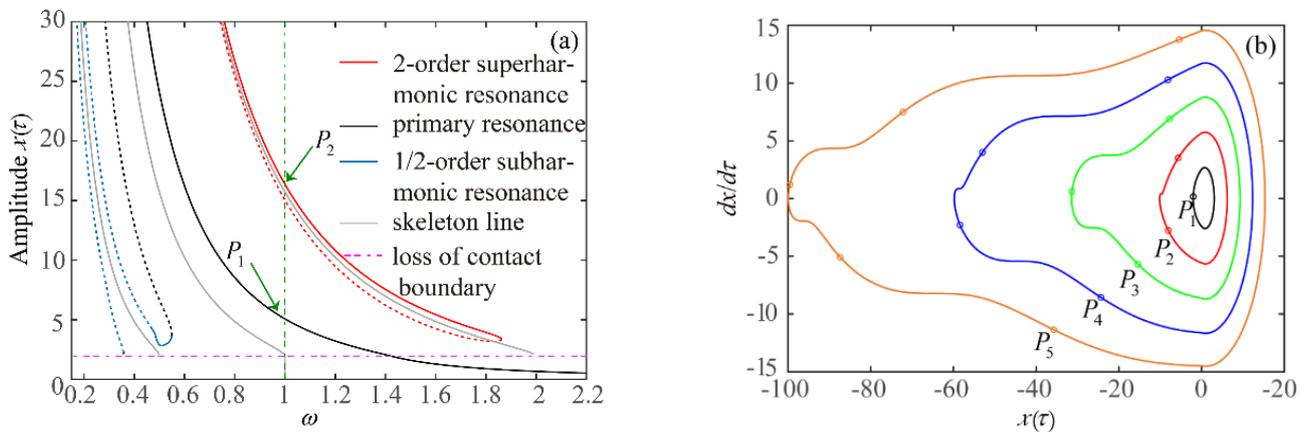
**Figure 9.** One-sided contact system for  $A = 1$ , (a) the frequency-response peak-to-peak curves, and (b) phase portraits their Poincare mapping dots of co-existing period- $n$  solutions (i.e.,  $P_n$ ) when  $\omega = 1$ .
