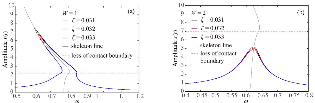
**Figure 7.** For  $\alpha = 0.6$ , influence of  $\zeta$  on the frequency-response peak-to-peak curves of one-sided contact system, (a)  $W = 1$  and (b)  $W = 2$ .
