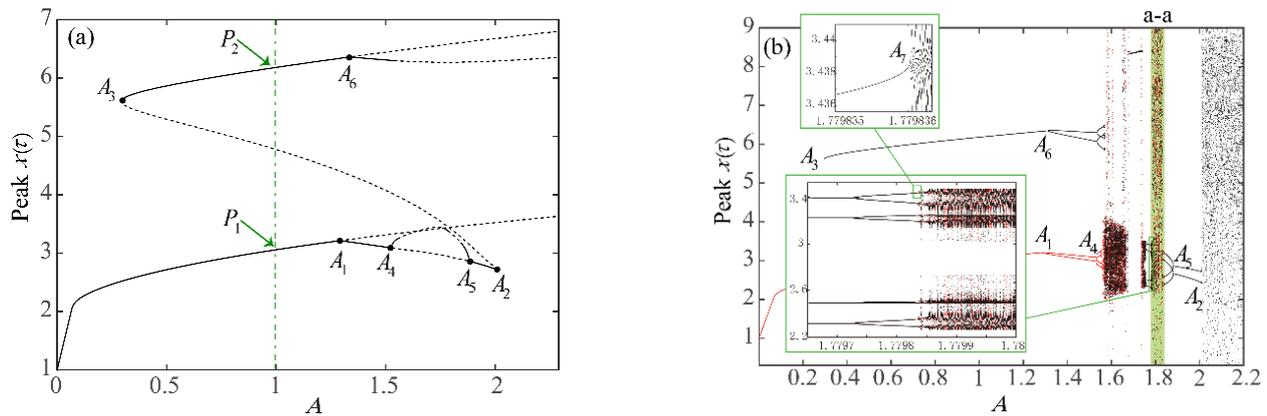
**Figure 8.** One-sided contact system for  $\omega = 1$ , (a) the periodic solution branch as the excitation amplitude  $A$  varies, and (b) numerical bifurcation diagrams of  $x(\tau)$  when  $A$  sweeps up (black dots) and down (red dots).
