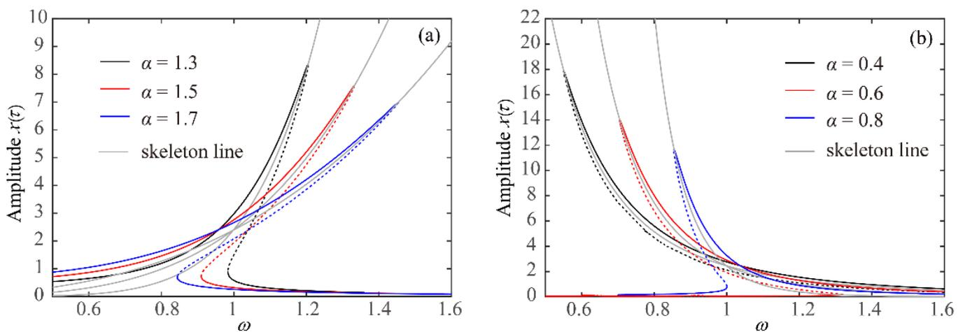
Figure 3. For  $W = 0$ , influence of  $\alpha$  on the frequency-response peak-to-peak curves of continuous system, (a)  $\alpha > 1$  and (b)  $0 < \alpha < 1$ .
