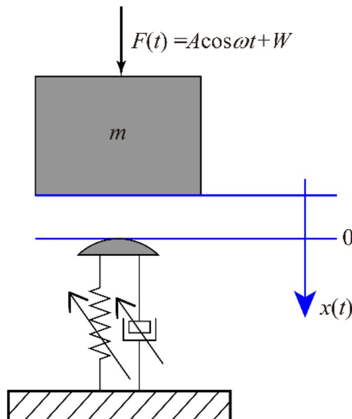
Figure 1. Power-form nonlinear one-sided contact system.
