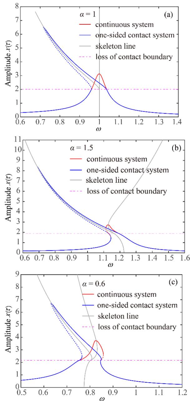
**Figure 5.** Comparisons of frequency-response peak-to-peak curves between continuous system and one-sided contact system, (a)  $\alpha = 1$ , (b)  $\alpha = 1.5$ , and (c)  $\alpha = 0.6$ , where the magenta dash line denotes the loss contact boundaries.
