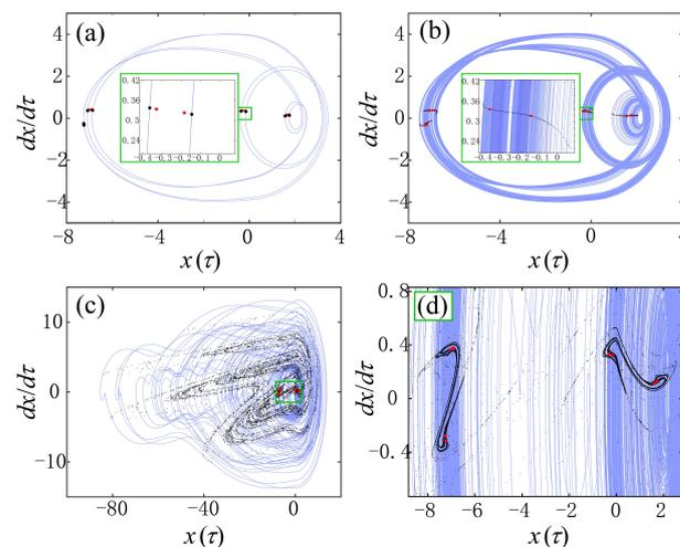
**Figure 11.** Phase portraits and their Poincaré mappings of one-sided contact system for  $\omega = 1$ , (a)  $A = 1.7798$ , (b)  $A = 1.78$ , (c)  $A = 1.785$ , and (d) the enlargement of (c), where the red dots denote the Poincaré mapping of unstable period-8 motion at  $A_7$  point (see Figure 8).
