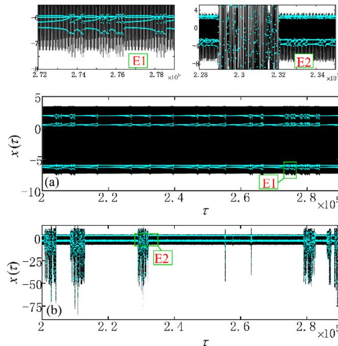
**Figure 10.** Time series  $x(\tau)$  and their enlargements of one-sided contact system for  $\omega = 1$ , (a)  $A = 1.78$ , and (b)  $A = 1.785$ , where the cyan dots denote the period-1 mapping points of  $x(\tau)$  at intervals of excitation period  $2\pi$ .
