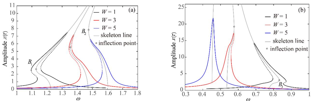
**Figure 4.** Influence of normal load  $W$  on  $\alpha$  the frequency-response peak-to-peak curves of continuous system, (a)  $\alpha = 1.5$  and (b)  $\alpha = 0.6$ .
