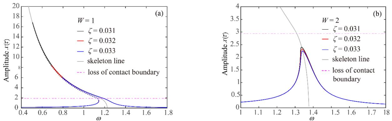
**Figure 6.** For  $\alpha = 1.5$ , influence of  $\zeta$  on the frequency-response peak-to-peak curves of one-sided contact system, (a)  $W = 1$  and (b)  $W = 2$ .
