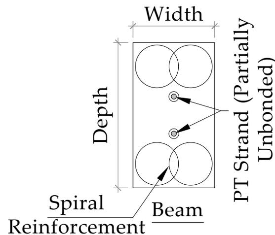
Figure 22. Spiral reinforcement at the compression zones.
