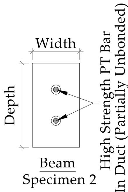
Figure 15. PT bar (partially unbonded).
