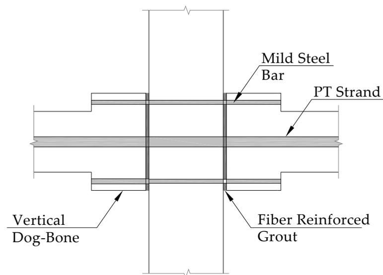
Figure 17. Precast column beam assembly with vertical dog bones.
