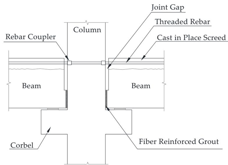
Figure 2. Cast-in-situ structural screed with a gap joint [26].
