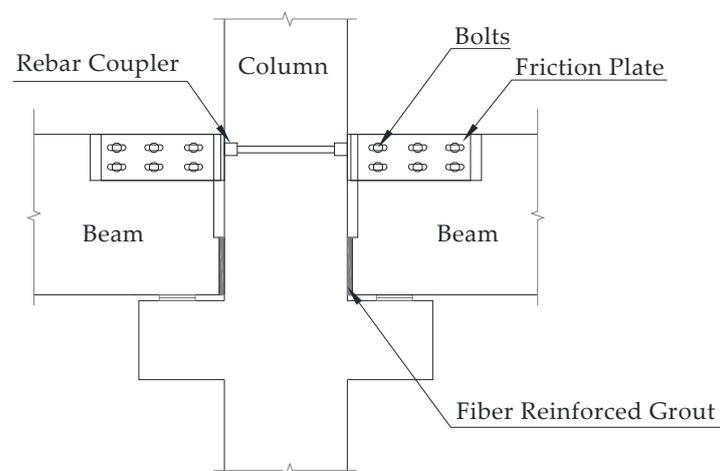
Figure 3. Example of connection with friction plates [26].
