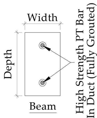
Figure 10. PT bar (fully grouted).
