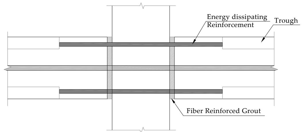
Figure 19. Precast beam column assembly.
