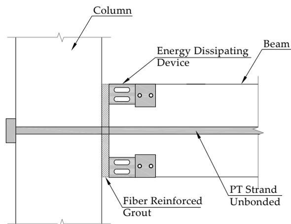
Figure 27. Proposed precast post-tensioned beam-column connection [49].
