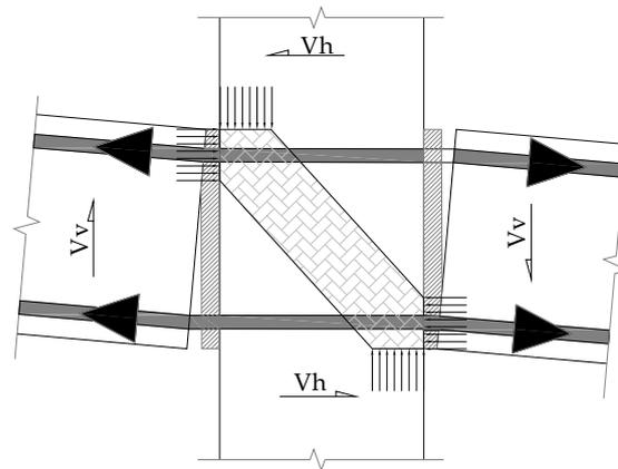
Figure 21. Shear transfer by the diagonal compression strut.
