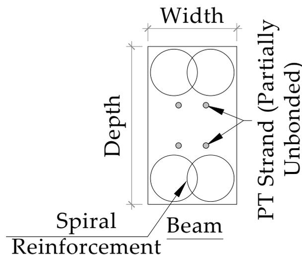
Figure 13. PT strand placed closer to the center and partially unbonded.
