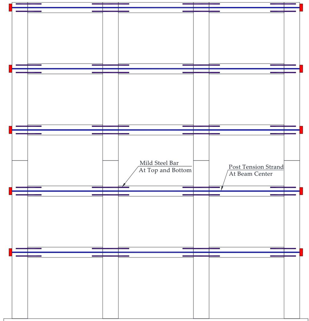
Figure 6. Precast hybrid frame [27].
