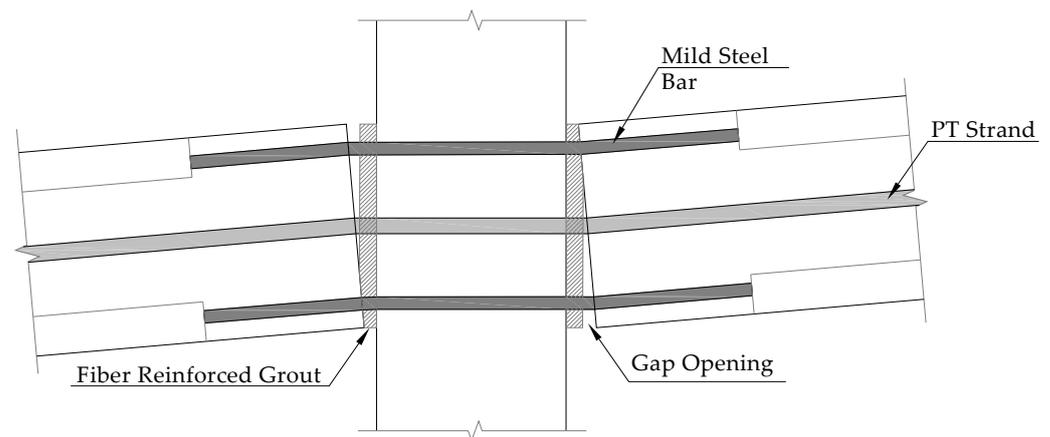
Figure 8. Deformed hybrid connection [28].
