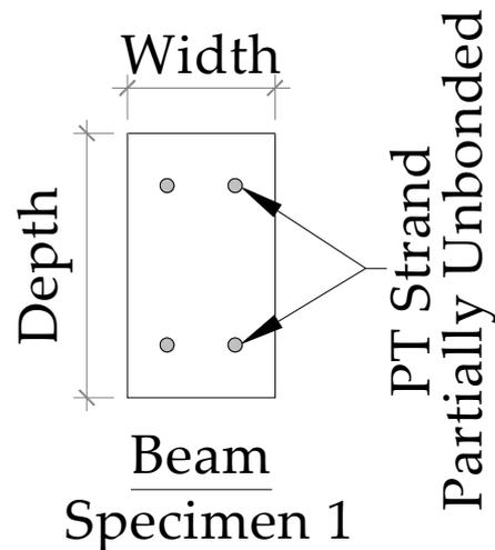
Figure 14. PT strand (partially unbonded).
