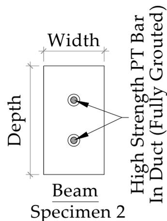
Figure 12. PT bar placed closer to the center and fully grouted.
