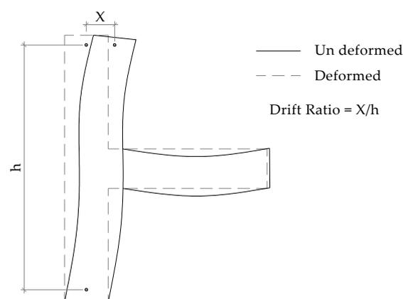
Figure 9. Drift ratio calculation as per ACI 374.1-05 [29].
