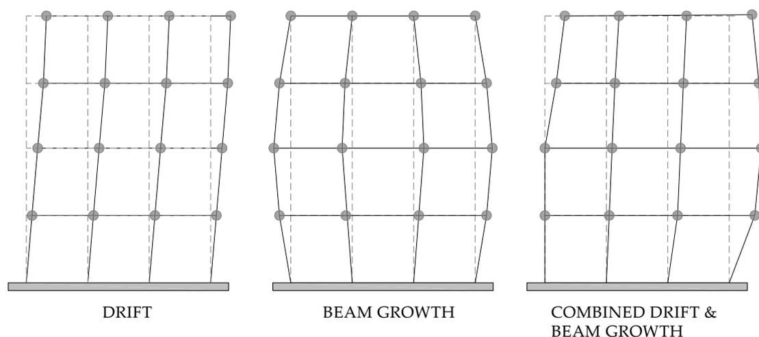
Figure 23. Frame sway including beam growth [46].
