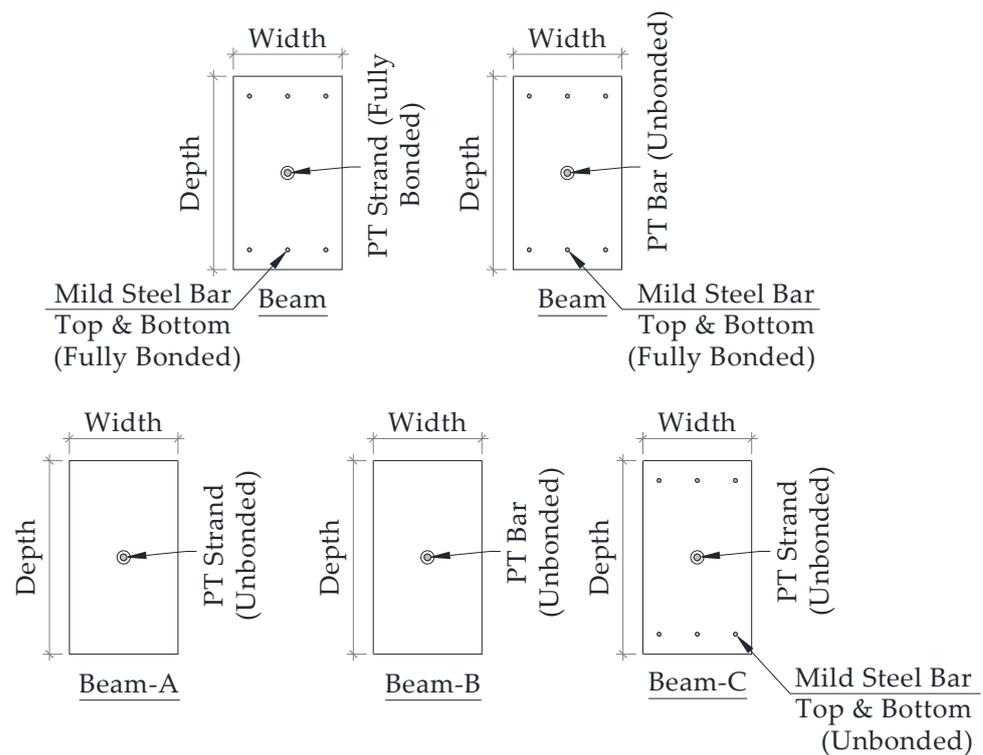
Figure 18. Five test specimens with various variables.
