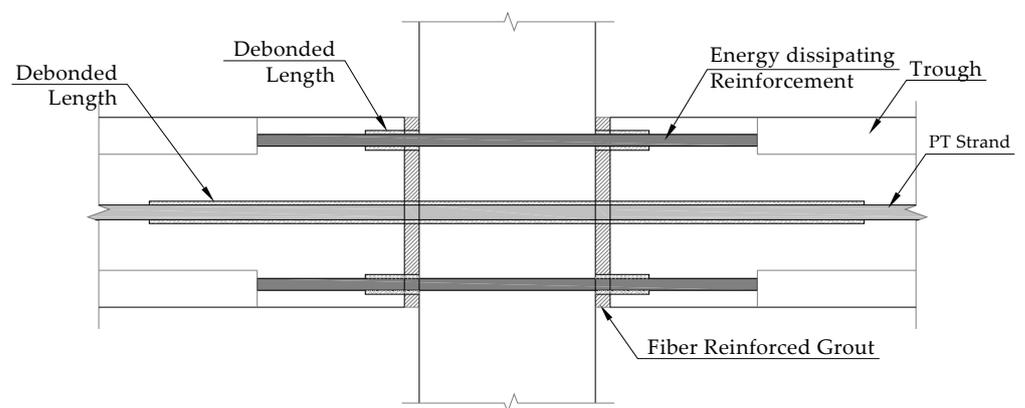
Figure 7. Undeformed hybrid connection [27].
