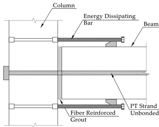
Figure 26. Proposed precast post-tensioned beam-column connection [50].
