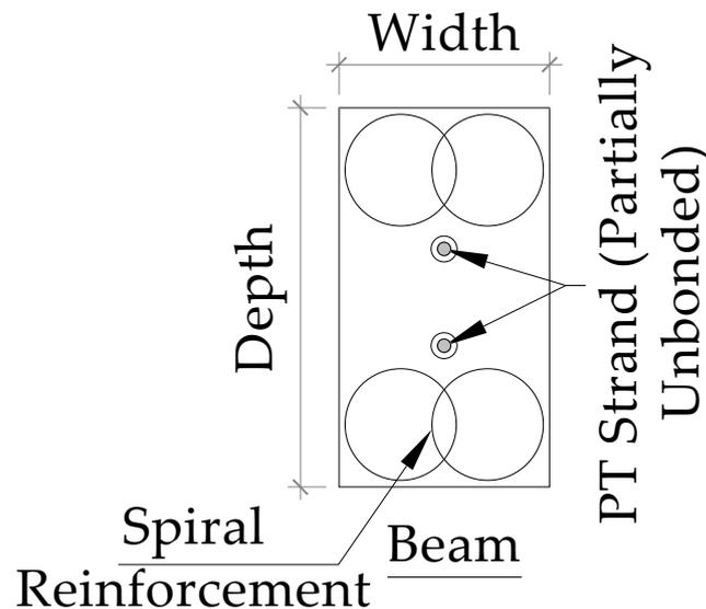
Figure 16. PT strand placed closer to the center and partially unbonded.
