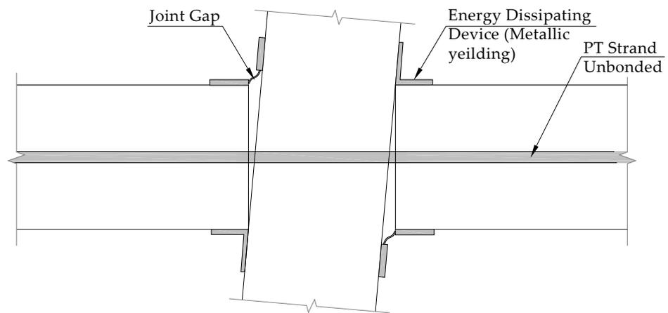
**Figure 29.** The proposed precast post-tensioned beam column connection (deformed) [54].
