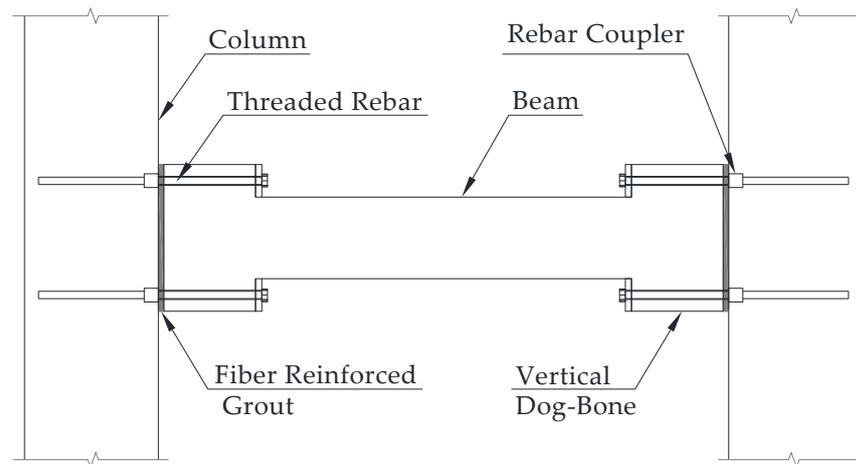
Figure 1. Vertical dog bones with threaded rebar [26].
