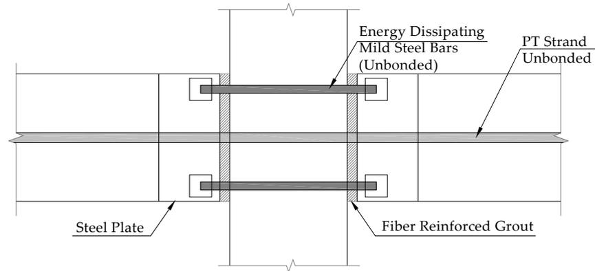
Figure 25. Proposed precast post-tensioned beam-column connection [48].
