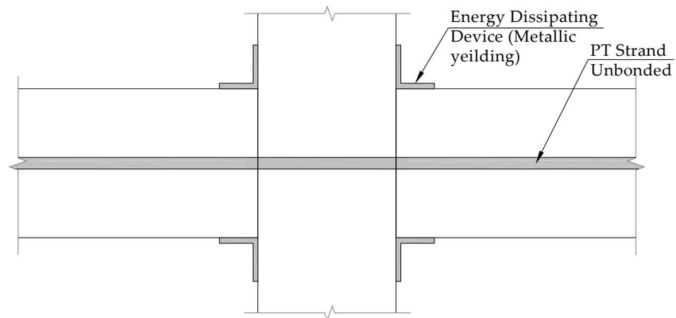
**Figure 28.** The proposed precast post-tensioned beam column connection (undeformed) [54].
