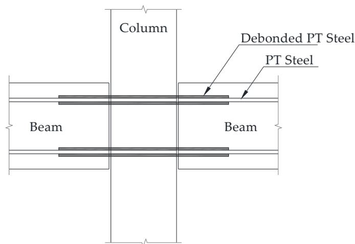
Figure 5. PT connection with unbonded strands [26].
