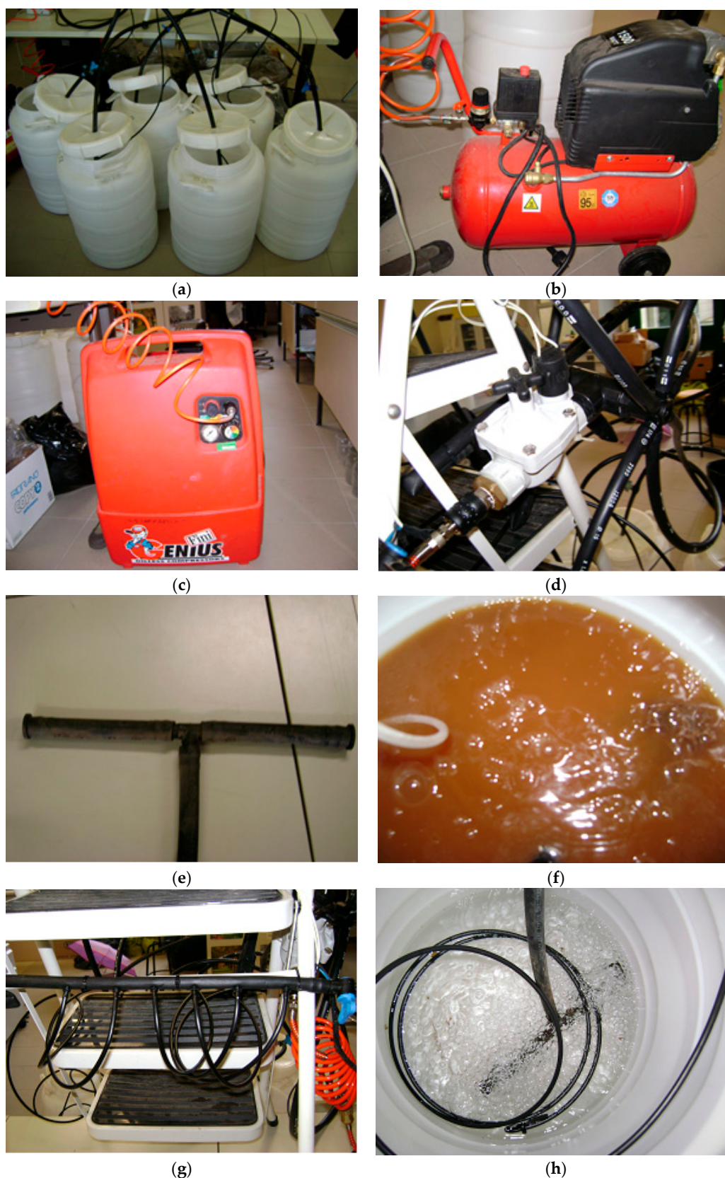
Scheme 1. Technical and operative details of the CT extraction process. (a) 50 L-plastic containers; (b) 24 L compressor; (c) 5 L compressor; (d) solenoid valve supplied with 24 V; (e) T-shaped end; (f) turbulence effect; (g) air-distributor made up of 6-mm pipes connected to a main 16-mm pipe by adapters; (h) spiral arrangement of the smaller tubes ( \varnothing 6 mm) in the container and sparkling effect.
