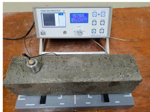
**Figure 2.** Measurement process of RDME.
