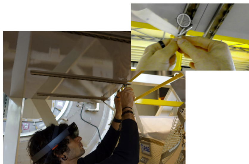
Figure 11. TSR installation in a physical mock-up of an ISS module using an AR system [68].
