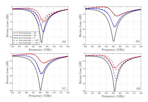
Figure 5. (a) Active return loss of Element #1 for varying steering angles, (b) active return loss of Element #2 for varying steering angles, (c) active return loss of Element #3 for varying steering angles, (d) active return loss of Element #4 for varying steering angles of radiating elements.
