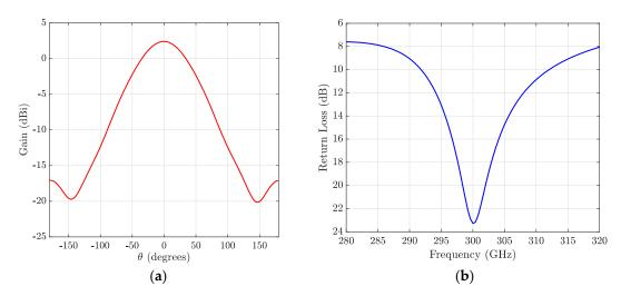
Figure 3. (a) Gain of unit cell, (b) return loss of unit cell.
