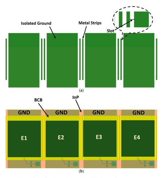
**Figure 8.** (a) Modified defected ground plane, (b) modified layout of  $1 \times 4$  array.
