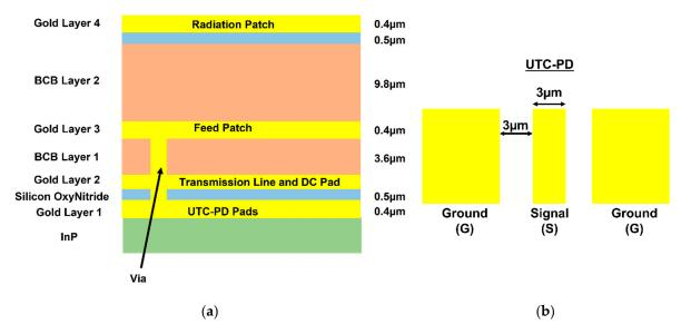
Figure 1. (a) Proposed epitaxial layer stack-up of InP, (b) pad dimensions of UTC-PD.
