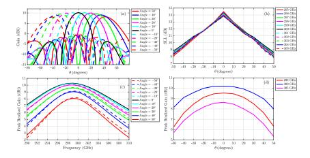
**Figure 10.** (a) Steering pattern for  $1 \times 4$  array at 300 GHz, (b) SLL of array, (c) peak realised gain vs. frequency for varying steering angles, (d) peak realised gain vs. steering angle for different frequencies.
