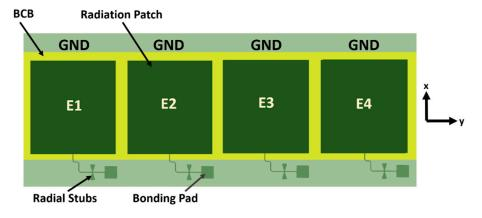
**Figure 4.** Top view of the designed  $1 \times 4$  antenna array.
