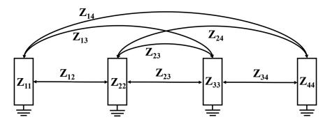
**Figure 7.** Impedance model of  $1 \times 4$  array.
