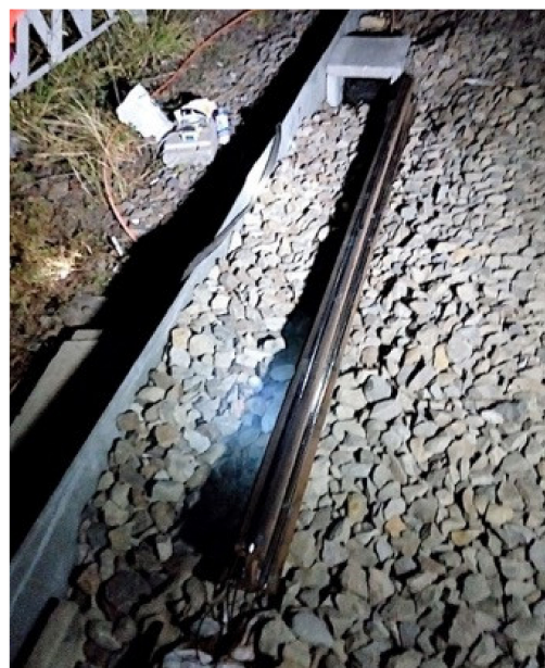
Figure 5. The reference track: this reference track was placed at mile 26K101 and was kept 2 m away from and parallel to the tested rail in the field.
