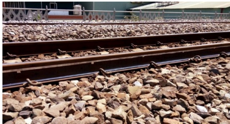
Figure 4. The sensing fibers after the installation: this picture was taken at mile 26K125 in the test field. To protect against fiber breakage from the impact of ballasts, all sensing fibers were covered by aluminum tape.
