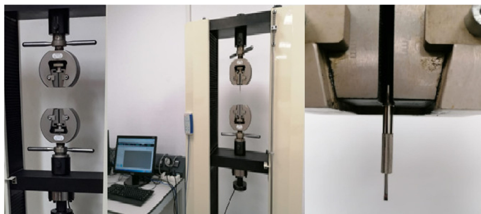
Figure 2. Device used for evaluation of the force required to detach the brackets.
