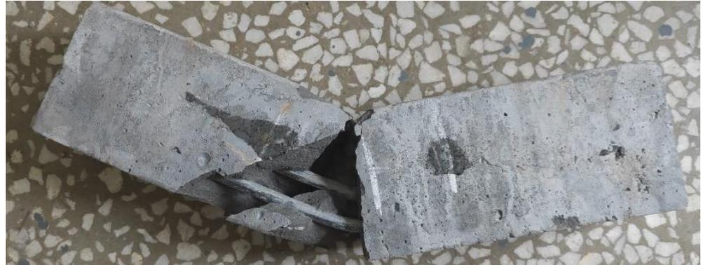
**Figure 6.** The failure state of SBRPC.
