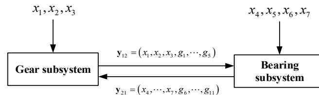
Figure 9. The coupling relationship diagram of speed reducer.
