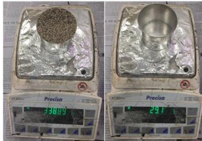
Figure 8. Equipment for determining relative density.
