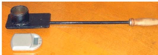
**Figure 2.** Soil bulk density measuring kit.
