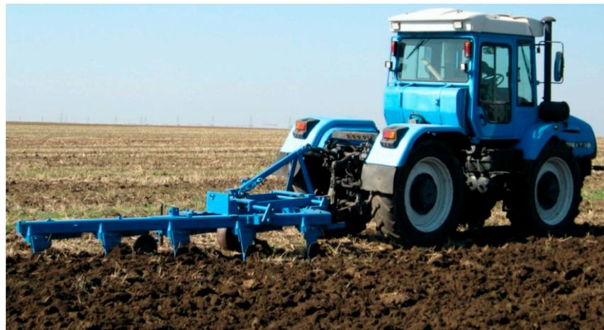
Figure 3. Tractor HTZ-17021 with five-furrow plow.
