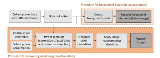
Figure 6. Overview of the attack proposed by Wei et al. [19] (artwork reworked).
