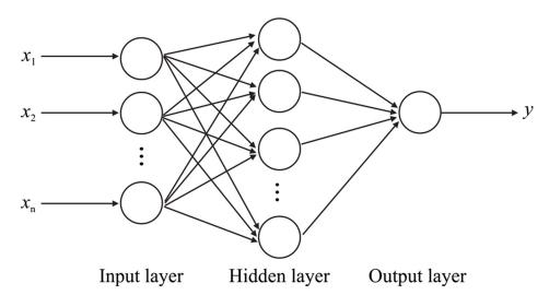
**Figure 1.** Multi Layer Perceptron, where *x* is the input and *y* is the output of a neuron.
