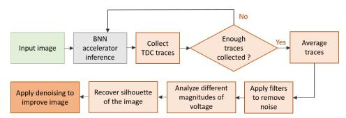
Figure 7. Overview of the attack proposed by Moini et al. [19] (artwork reworked).
