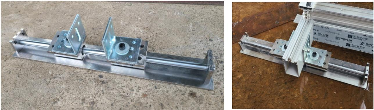
Figure 5. Seismic fastener prototype (X-axis).
