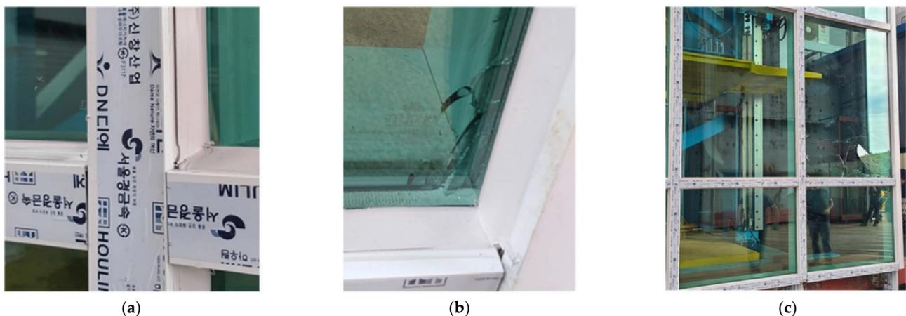
**Figure 13.** States of non-seismic curtain wall after the dynamic racking crescendo test: (a) silicone cracks (42 mm); (b) glass cracks (60 mm); (c) glass fallout (90 mm).
