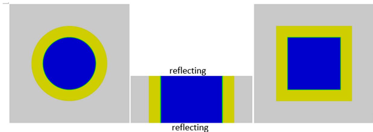
**Figure 5.** The general 2-D (left and centre) Monte-Carlo model of the configuration (left, top view x-y, centre front view x-z) and 3-D (left and right) Monte-Carlo model of the configuration (left, top view x-y, right front view x-z) with molten salt fuel core—blue, stainless steel vessel—light green, reflector—yellow, and vacuum—grey used for the validation of the results and the 3-D studies.
