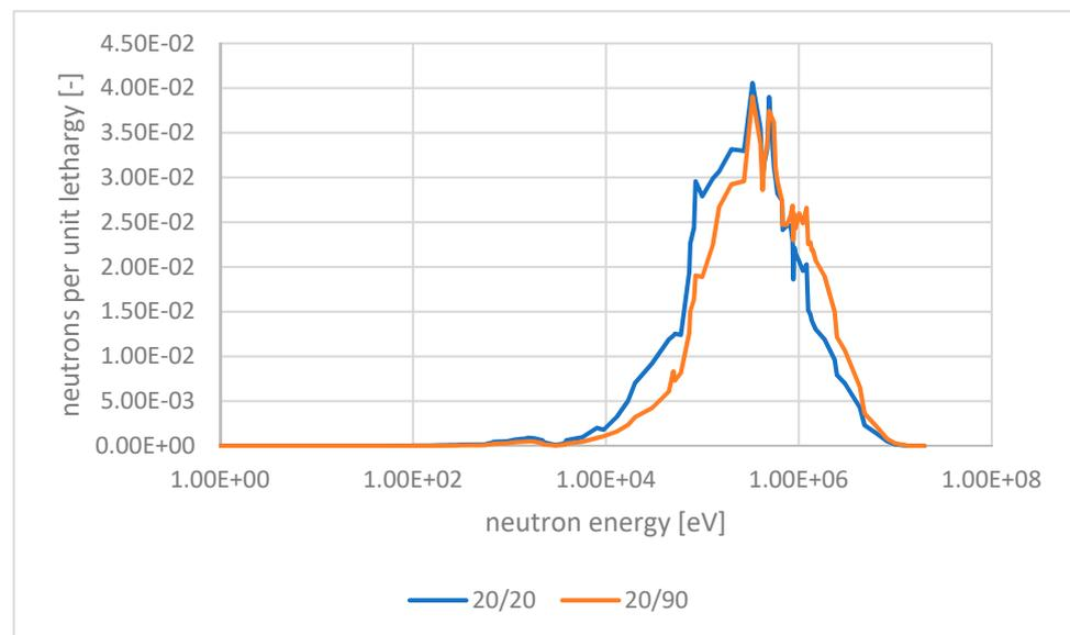
**Figure 11.** Neutron spectrum for the heavy metal rich system (20% NaCl) with 20% enrichment (20/20) compared to the 90% enriched system (20/90) (calculated through POLARIS).
