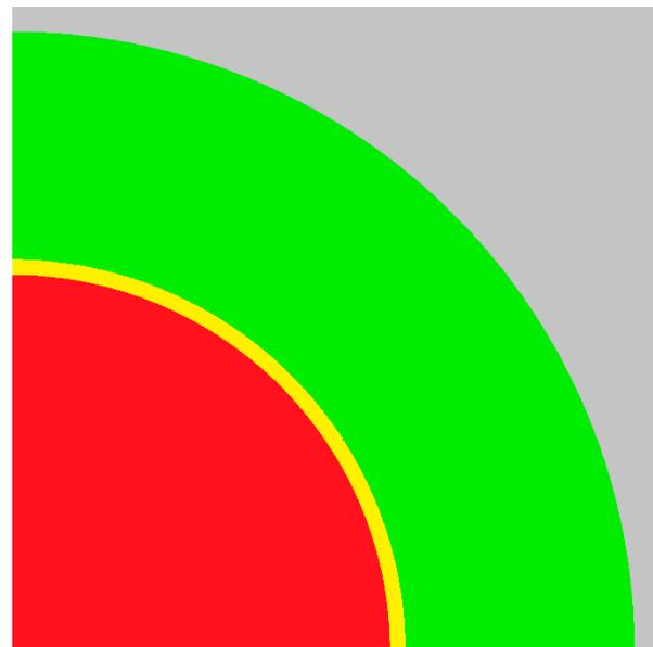
**Figure 4.** The 2-D SCALE/TRITON-NEWT model (molten salt fuel core—red, stainless steel—yellow, NaCl reflector—light green, vacuum—grey) used for the analysis of the neutron flux distribution.
