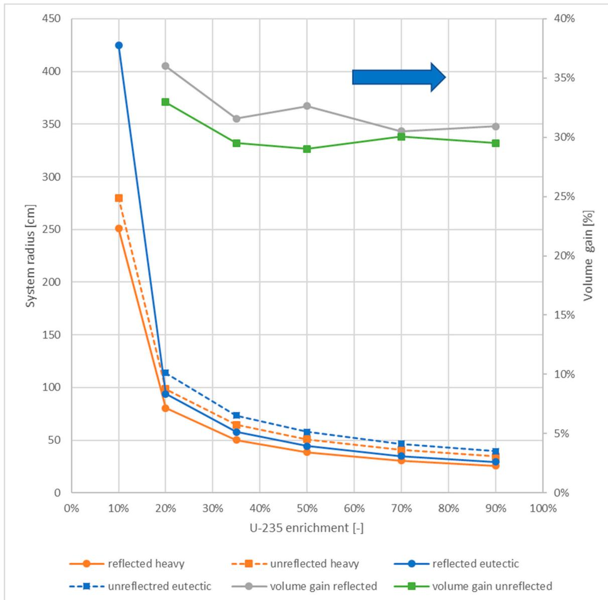
**Figure 6.** 2-D system radius for the eutectic and the heavy metal rich system depending on uranium enrichment for the reflected and the unreflected systems as well as the volume gain per step archived by changing from the eutectic to the heavy metal rich system (calculated through POLARIS).
