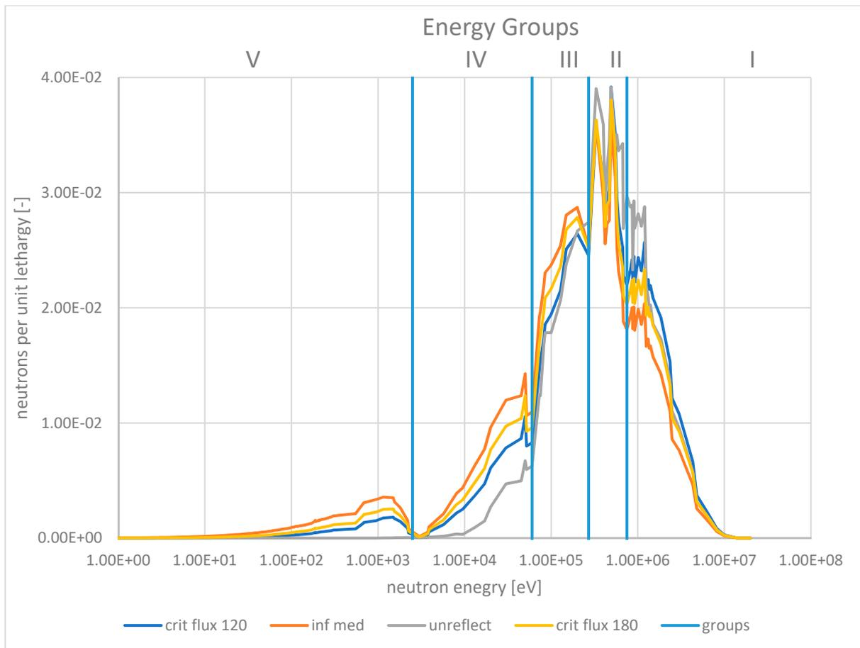
**Figure 12.** Neutron flux spectrum for the reflected and the unreflected core as well as for different axial leakage approximation (infinite medium, 120 cm core height, and 180 cm core height) using different core heights with added neutron group structure for the spatial flux distribution analysis.
