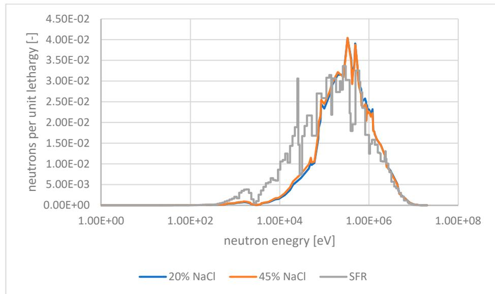
**Figure 9.** Integral neutron spectrum 35% enriched for the eutectic and the heavy metal rich system in comparison with the neutron spectrum in a classical sodium cooled fast reactor (SFR) fuel assembly of EFR type (calculated through POLARIS, the SFR case is based on HELIOS [24]).
