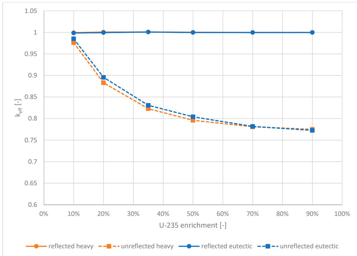
**Figure 7.** 2-D system criticality reduction by eliminating the reflector for the eutectic and the heavy metal rich system depending on uranium enrichment (calculated through POLARIS).
