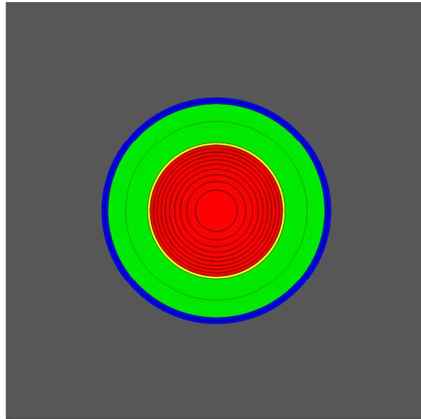
**Figure 3.** The 2-D SCALE/POLARIS model (molten salt fuel core—red, stainless steel—yellow, NaCl reflector—light green, vacuum—blue, absorber material—dark grey) used for the general analysis.
