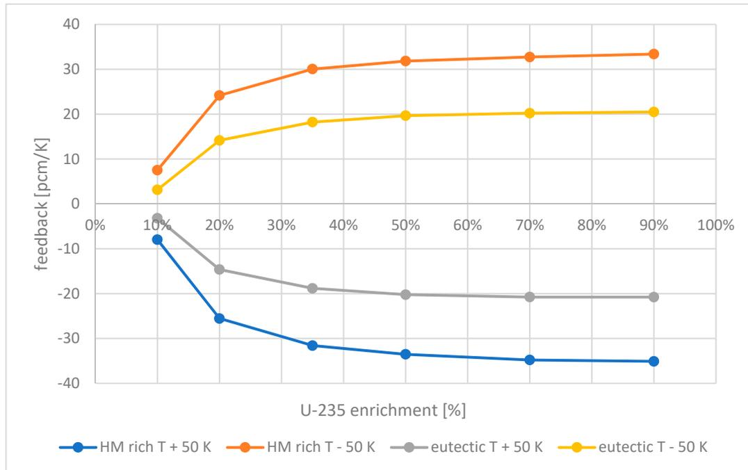
**Figure 8.** 2-D system thermal feedback effects (salt density and fuel temperature) for the eutectic and the heavy metal rich system depending on uranium enrichment (calculated through POLARIS).
