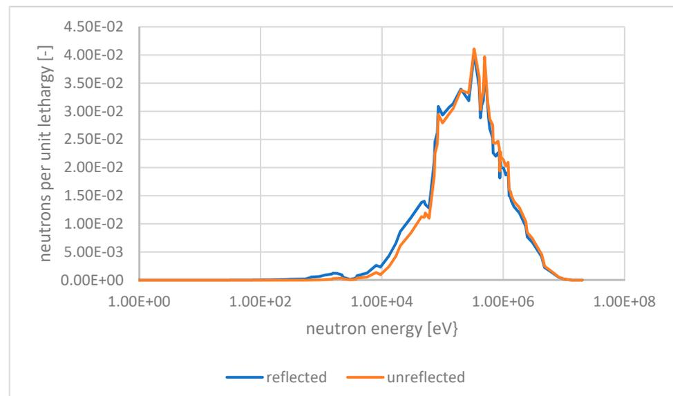
**Figure 10.** Neutron spectrum 20% enriched for the reflected and reflected eutectic system (calculated through POLARIS).
