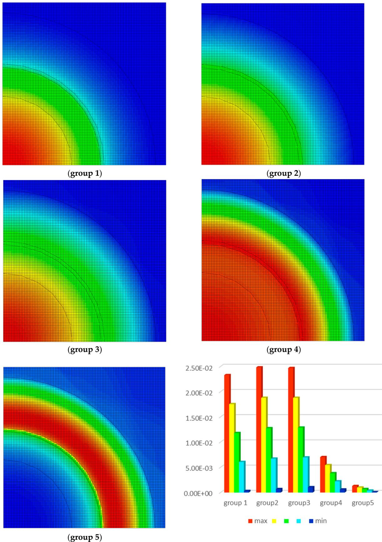
**Figure 13.** Spatial neutron flux distribution in the 5 energy groups defined in Figure 12 and related neutron flux values in each group with the colour map given in the bottom right figure (calculated using a TRITON-NEWT sequence).
