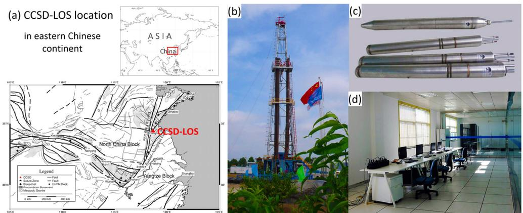
**Figure 1.** The CCSD long-term crustal movement observation station (CCSD-LOS). (a) The location of the station in China; (b) the observation borehole of the CCSD-LOS. The picture shows the derrick and drill pipes for the installation of instruments, with a 5158 m-deep hole below; (c) some underground probes installed in the boreholes. They have now been installed in 4 layers underground; and (d) the supervisory control room.
