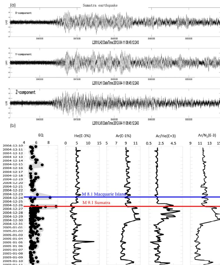
**Figure 3.** (a) A 3-component record of Sumatra earthquake observed. (b) Real-time gas anomalies observed during the CCSD drilling; the vertical ordinate is the date of observation; columns from the left to right are the seismic magnitude, records of helium, argon, argon/helium, and argon/nitrogen, respectively.
