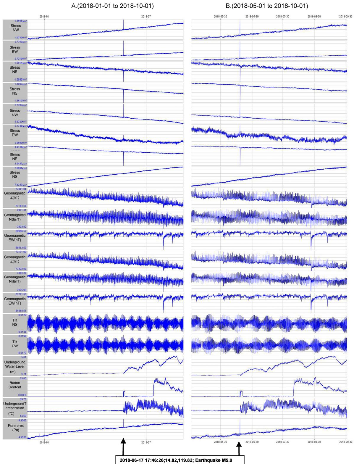
**Figure 4.** Records of underground monitoring parameters before and after the Philippine magnitude-5 earthquake. The monitoring parameters from the top to the bottom are as follows: the in situ stress components of eight azimuths, geomagnetic field components of six azimuths, the earth tilt components of two azimuths, underground water level, gas radon content, underground formation temperature and pressure, and pore pressure.
