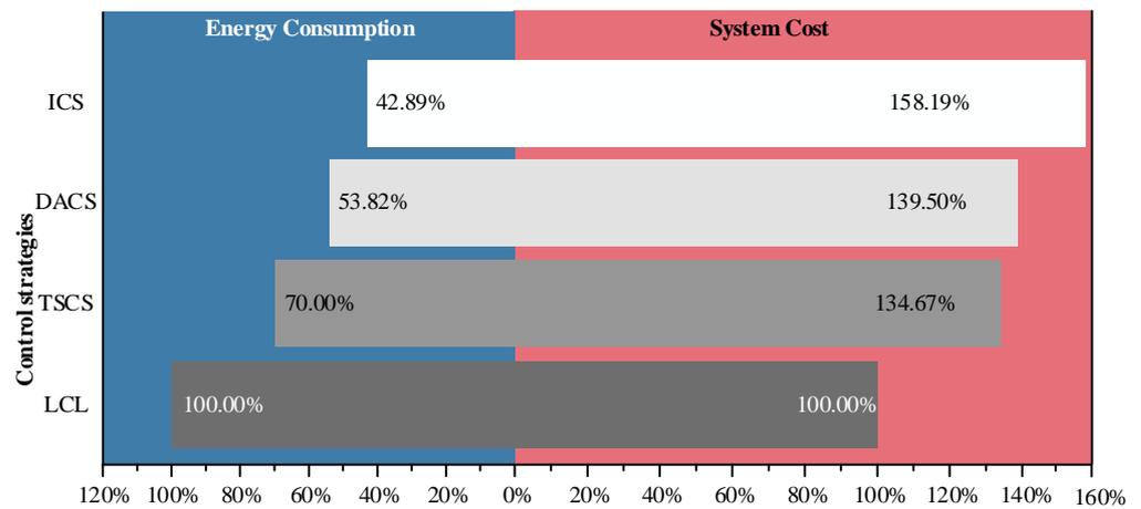
Figure 4. Relationship between control strategy and energy consumption/system cost.
