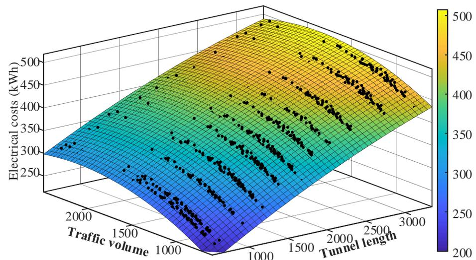
**Figure 9.** Electrical costs of a tunnel lighting system versus traffic volume and tunnel length for the ICS strategy.
