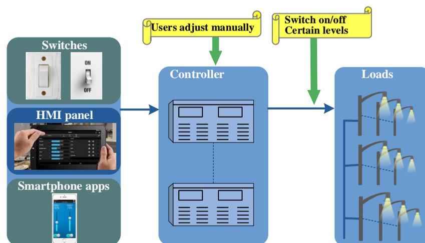
Figure 1. Manual control scheme.
