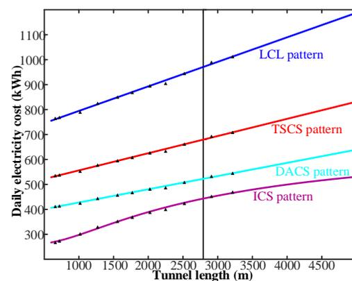
**Figure 8.** Energy consumption versus tunnel length for the four control strategies.
