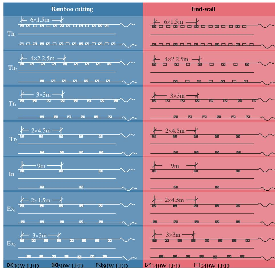
Figure 7. Lamps' installation rules for study tunnels.
