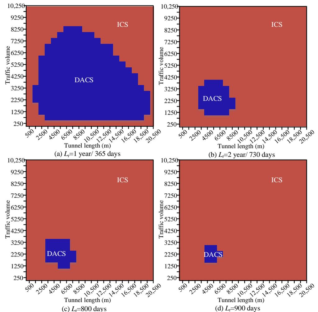
Figure 10. Choice of the control strategy for tunnels with different traffic volumes and lengths.
