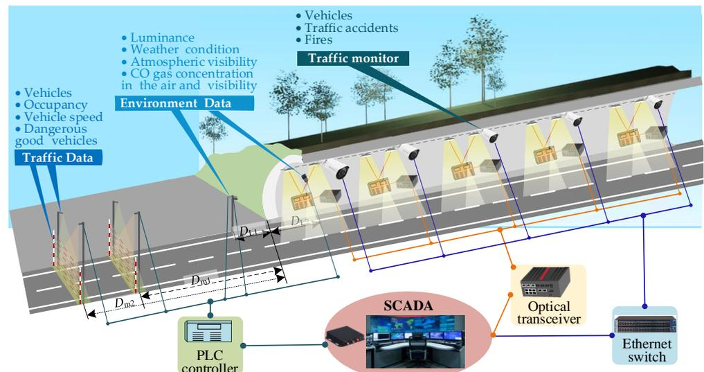
Note: *D<sub>m2</sub>* (700 m) and *D<sub>m1</sub>* (600 m) indicate the distance between the tunnel entrance and the microwave sets 1/2, and the microwave sets 3/4. *D<sub>L1</sub>*: Distance between luminance meter and tunnel entrance port (100 m). *D<sub>L2</sub>*: Distance between CO/VI detector and tunnel entrance port (200 m).
