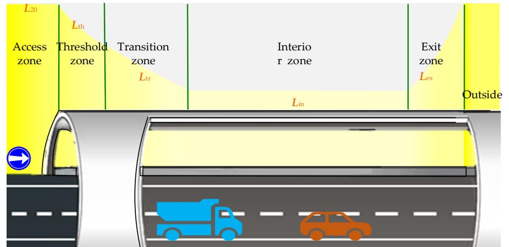
*Note:*  $L_{20}$  is the average luminance value measured in a  $20^\circ$  conical field of view defined at the SSD from tunnel entrance.  $L_{th}$ ,  $L_{tr}$ ,  $L_{in}$ ,  $L_{ex}$  are luminance of threshold zone, transition zone, interior zone and exit zone, respectively.
