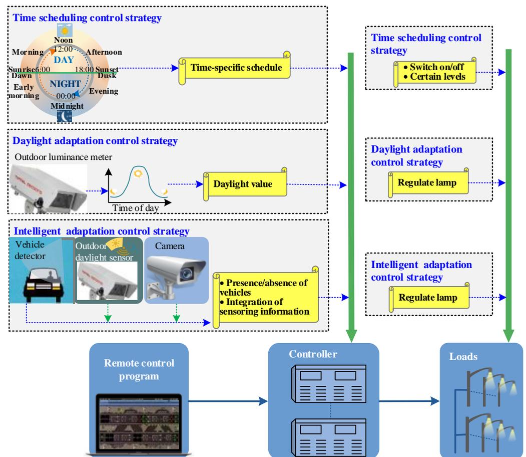
Figure 2. Time scheduling, daylight adaptation, and intelligent control schemes.
