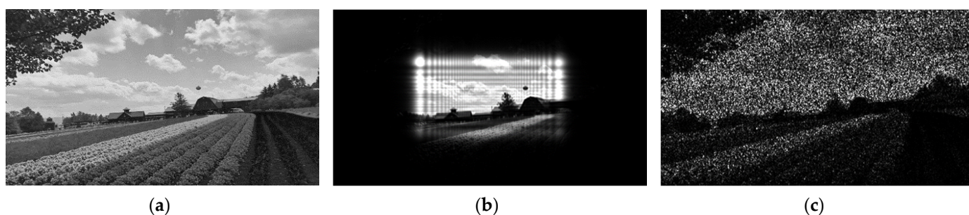
Figure 1. Original and simulated reconstructed images: (a) original image, (b) reconstructed image without random phase, (c) reconstructed image with random phase.
