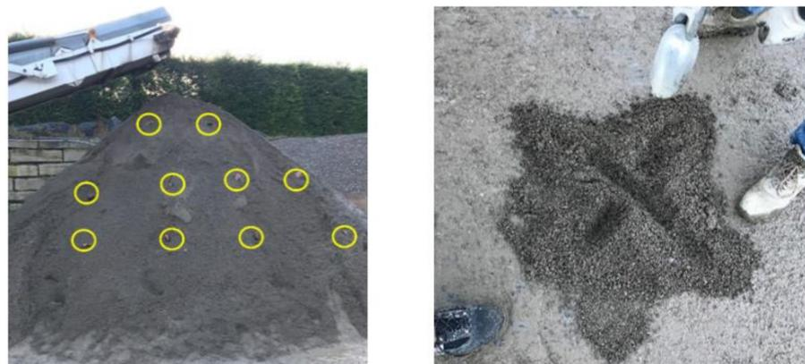
Figure 2. RA sampling points and quartering operation.
