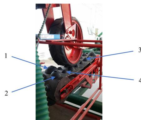
**Figure 8.** Seed meter drive belt provided with rubber hemispheres: (1) hemispheres with  $\Phi 100 \text{ mm}$ ; (2) hemispheres with  $\Phi 80 \text{ mm}$ ; (3) hemispheres with  $\Phi 50 \text{ mm}$ ; and (4) hemispheres with  $\Phi 30 \text{ mm}$ .
