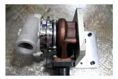
Figure 7. Oil-free turbocharger host machine by Hunan University [54].
