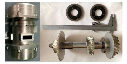
Figure 5. Airborne turbo cooler by Xi'an Jiaotong University [50].
