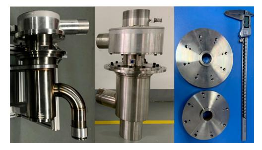
Figure 3. Helium turbo-expander and hydrogen turbo-expander by Xi'an Jiaotong University.
