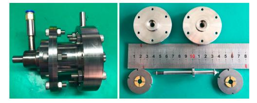
Figure 4. CO<sub>2</sub> turbo-expander by Xi'an Jiaotong University.
