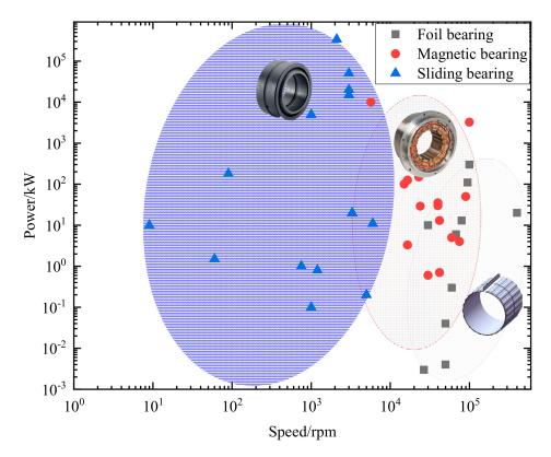
Figure 1. Application range of different kinds bearings.
