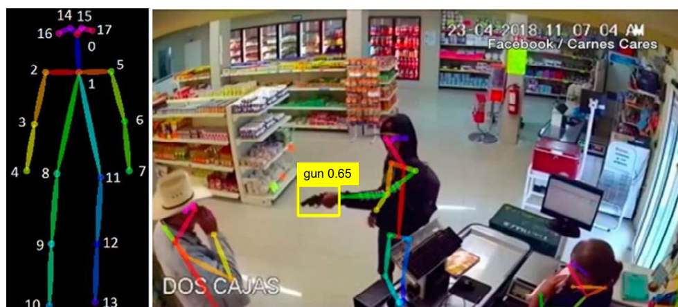
Figure 4. Pose skeleton composed of keypoints (left) and the calculation of pose skeletons using OpenPose in live images (right).
