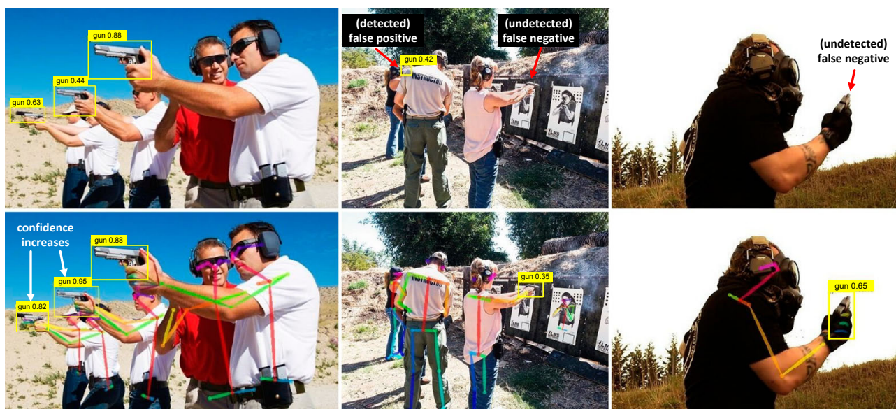
Figure 9. Results with YOLOv3 trained with the original image (top) and when trained with the image overlying the pose information (bottom).
