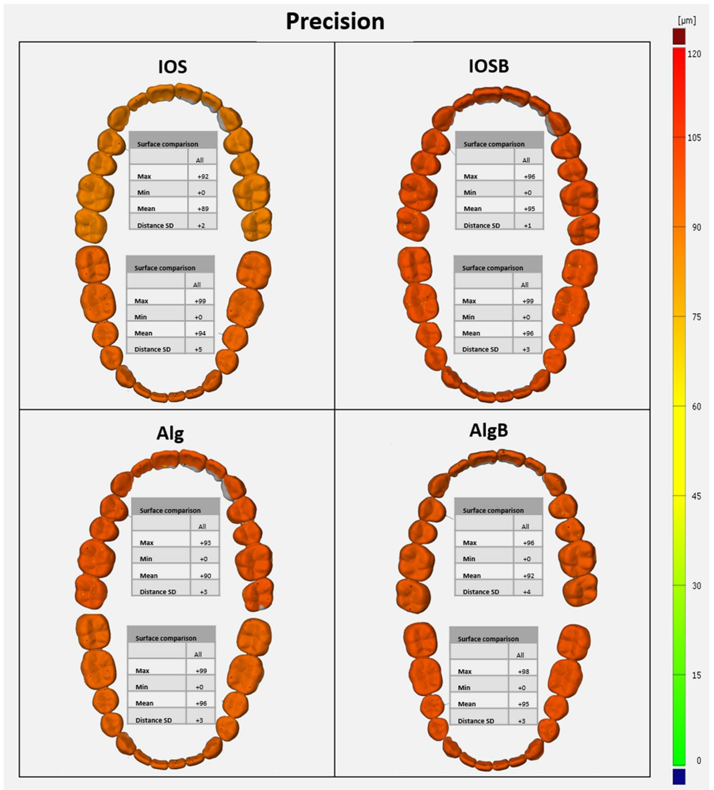
**Figure 6.** Color maps showing the precision assessment measured through the alginate impression and TRIOS3<sup>®</sup> intraoral scanners.
