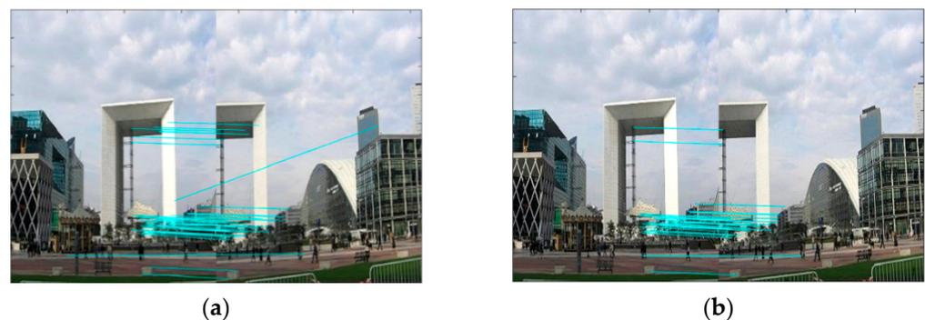
**Figure 8.** The registered images for T2: (a) I-RANSAC; (b) IIR. In complex scenarios, I-RANSAC mismatches, as shown in T2 (a), and IIR eliminates mismatches, as shown in T2 (b).
