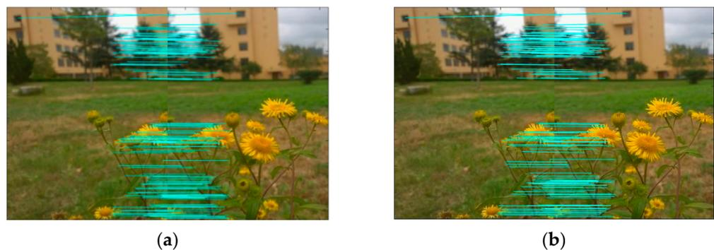
**Figure 7.** The registered images for T1: (a) I-RANSAC; (b) IIR. The blue line indicates the corresponding matching points of the two pictures. The registration accuracy of T1 (a) is 89.20%, and that of T1 (b) is 91.37%, as shown in Table 3.
