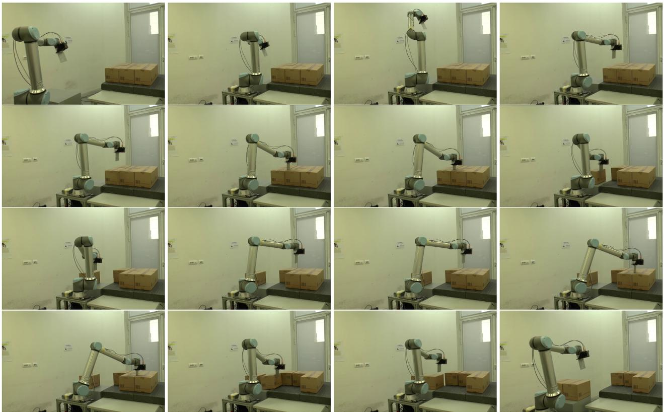
**Figure 7.** From top-left to bottom-right: a sequence showing the execution of a 2-boxes depalletizing task by the mobile manipulator.
