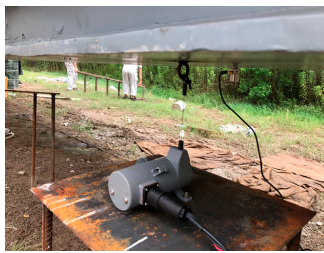
(a) Vertical vibration test on the suspension bogie
