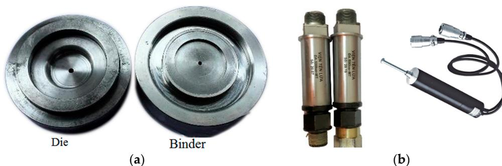
Figure 5. Components of the experimental system. (a) Hydrostatic die and binder (lower die); (b) Pressure sensors, stroke sensor.
