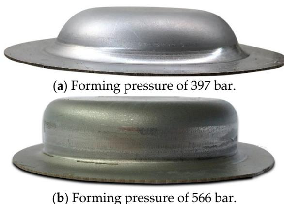
**Figure 7.** Products at different forming pressures.
