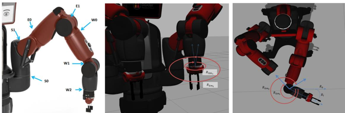
Figure 8. Configuration of the wrist joints: (left) Baxter joints; (center) standard configuration using W2 for Z-axis twist; (right) our configuration using W1 for Z-axis twist.
