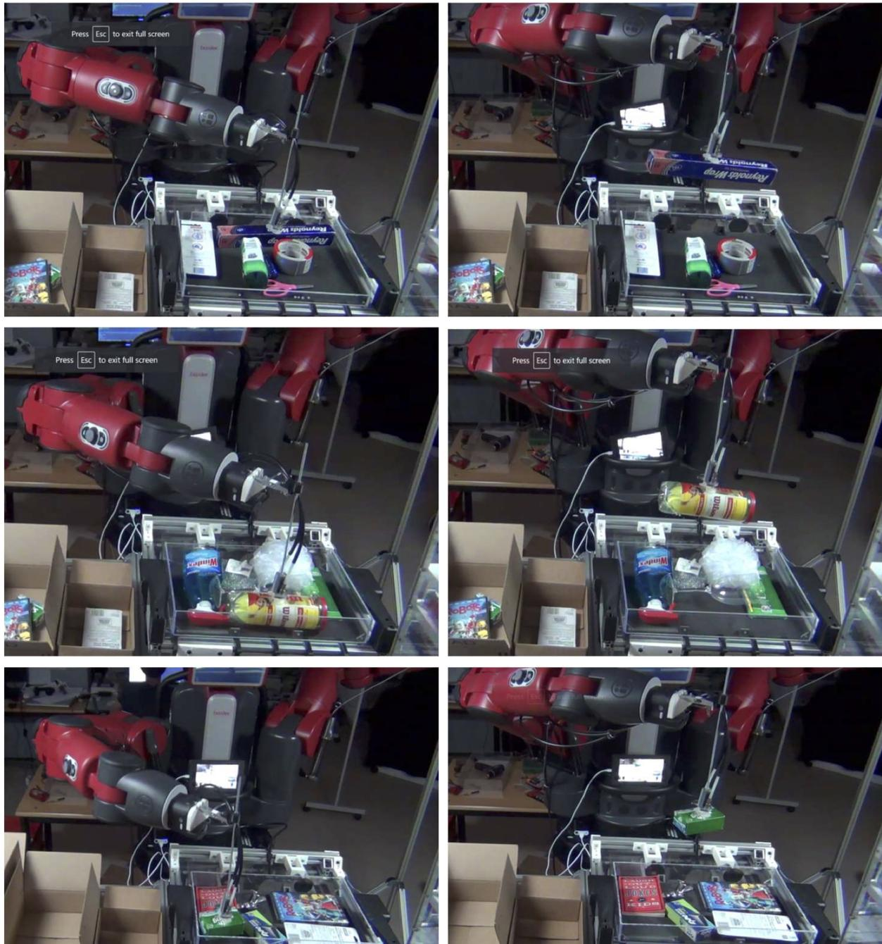
Figure 16. CNA with vacuum; successful grasp of the Reynolds' wrap, tennis ball container and Irish spring soap.
