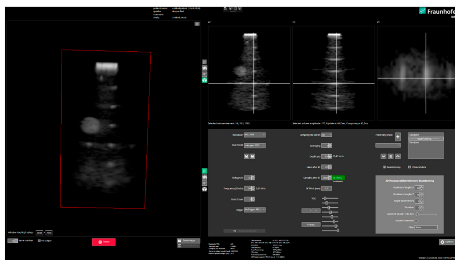
Figure 13. Real-time volumetric imaging user interface “USPilot” with device parameterization, volumetric rendering and orthogonal slice display.
