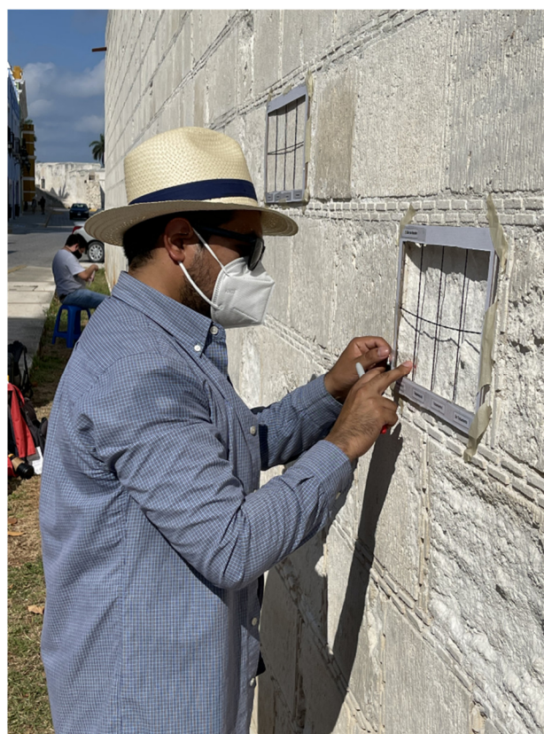
Figure 1. Limestone wall in Campeche, southern México, exhibiting a range of deterioration pathologies. Formers are being used to demarcate panels prior to treatment by spraying with carbonatogenic bacterial suspension or control solution. Replicate panels will allow statistical analysis. The aim is to increase surface hardness and reduce the detachment rate of flaking material.
