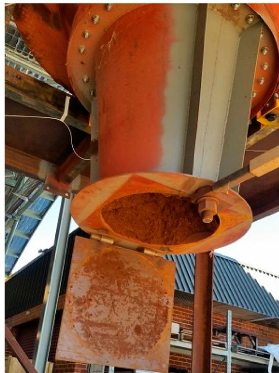
Figure 5. Blocked hopper.
