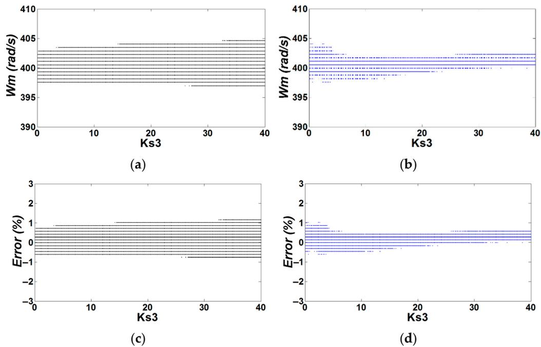
**Figure 8.** Bifurcation diagrams of the buck-motor system controlled with ZAD ( $K_{S1} = K_{S2} = 2 K_{S3} = 40$ , delay time  $166.6 \mu s$ , and quantization effects): (a)  $W_m$  vs.  $K_{S3}$  numerical, (b)  $W_m$  vs.  $K_{S3}$  experimental, (c) error vs.  $K_{S3}$  numeric, and (d) error vs.  $K_{S3}$  experimental.
