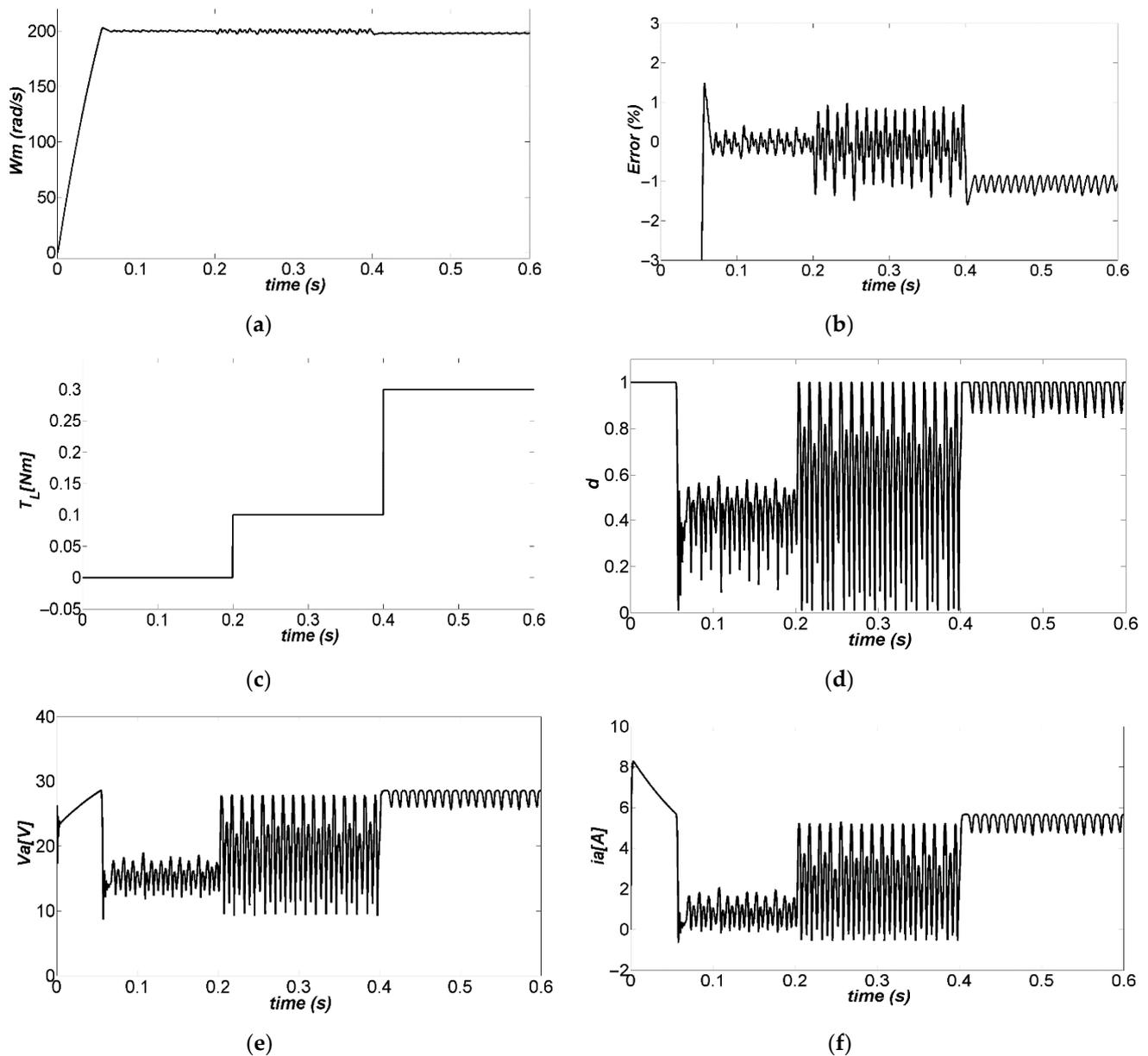
**Figure 10.** Simulation of the closed-loop system under varying load torque: (a) trajectory of the output, (b) trajectory of the output tracking error, (c) trajectory of the  $T_L$ , (d) trajectory of the  $d$ , (e) trajectory of the  $V_a$ , (f) trajectory of the  $i_a$ .
