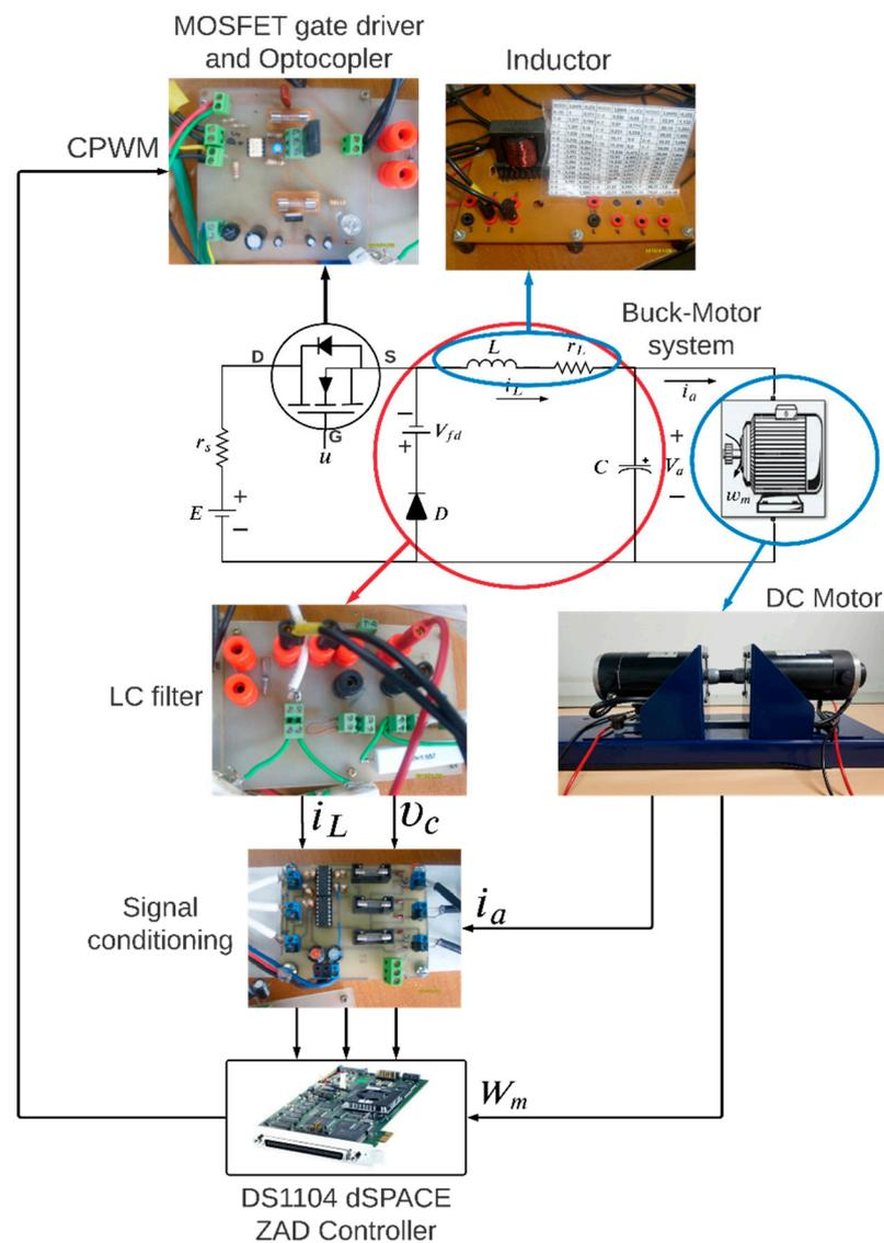
**Figure 6.** Experimental platform for validating the ZAD control.
