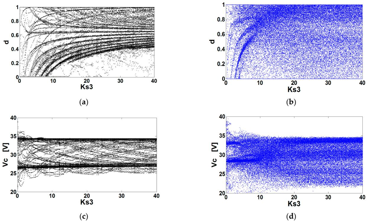
**Figure 9.** Bifurcation diagrams of the buck-motor system controlled with ZAD ( $K_{S1} = K_{S2} = 2 K_{S3} = 40$ , delay time  $166.6 \mu s$ , and quantization effects): (a)  $d$  vs.  $K_{S3}$  numerical, (b)  $d$  vs.  $K_{S3}$  experimental, (c)  $v_c$  vs.  $K_{S3}$  numerical, and (d)  $v_c$  vs.  $K_{S3}$  experimental.
