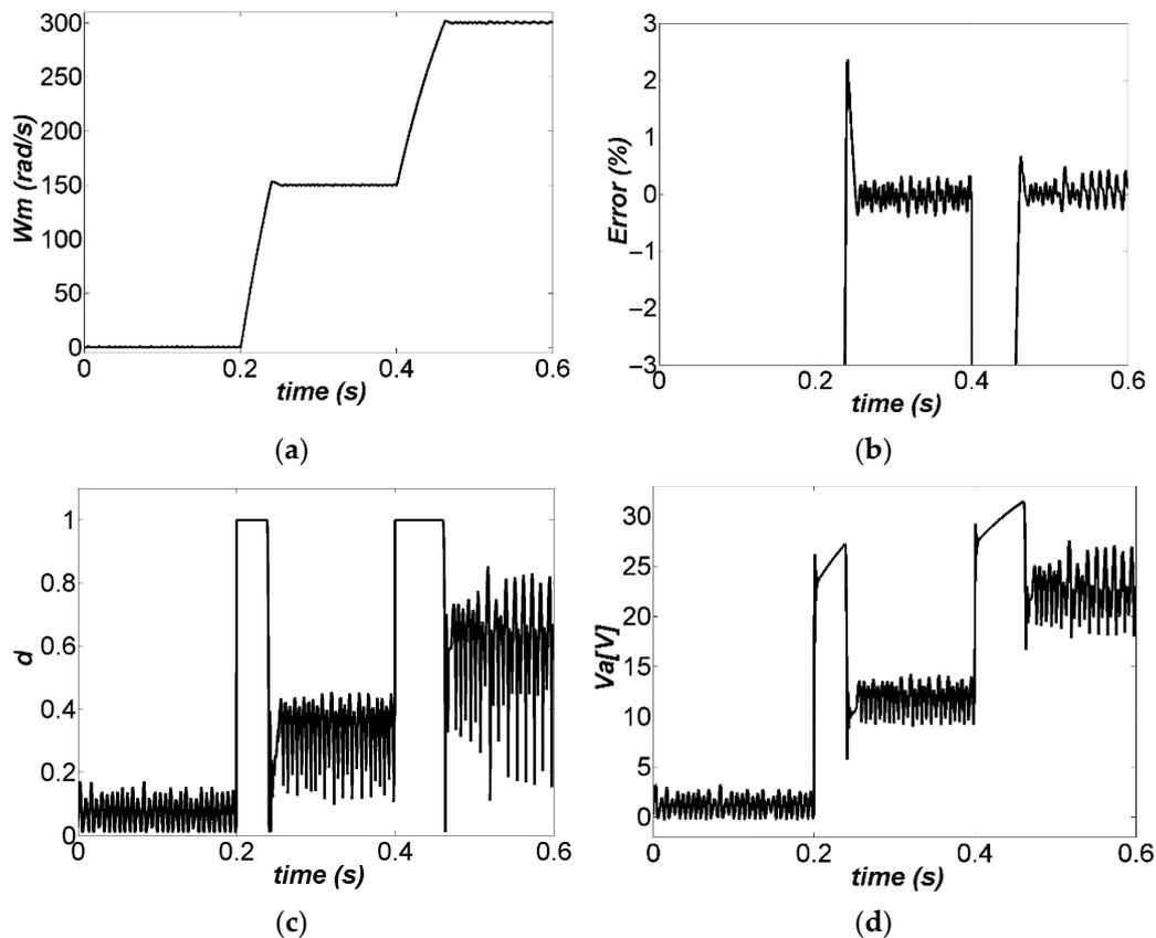
**Figure 7.** Output response for several reference signals,  $W_{mref} = 0$  rad/s;  $W_{mref} = 150$  rad/s;  $W_{mref} = 300$  rad/s: (a) Speed of the DC motor controlled, (b) Percentage of output tracking error, (c) Unsaturated duty cycle, (d) DC motor power supply.
