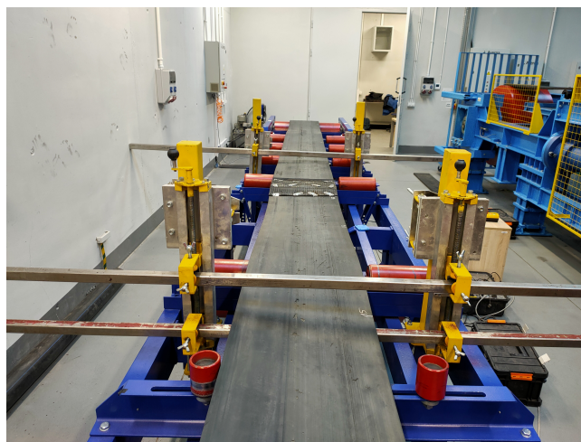
Figure 3. The device for non-invasive magnetic diagnostic of the belt.
