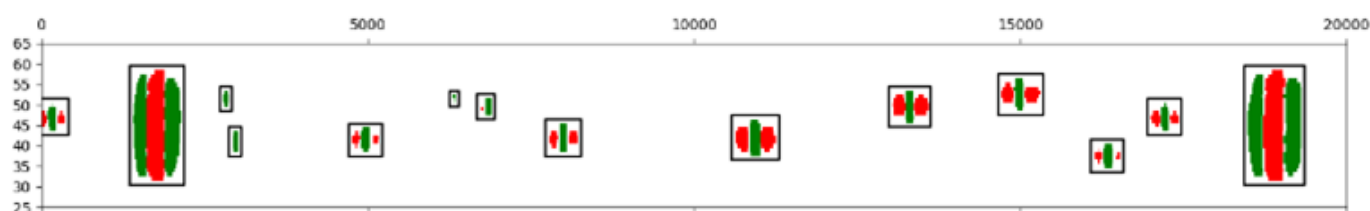
Figure 8. Representative conveyor belt—borders of potentially damaged areas.
