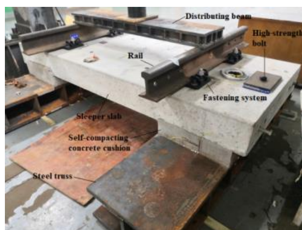
Figure 2. Model of rail–sleeper slab combined track structure.
