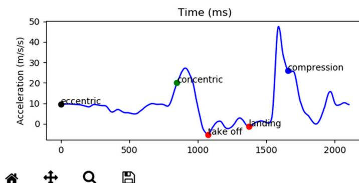
**Figure 13.** View of a processed jump showing the jumping metrics and the accelerometer graph.
