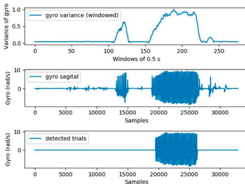
**Figure 7.** The running activity recognition algorithm. The figure in the middle depicts the input signal; the top figure shows the calculated variance in each of the 0.5 s windows in which the signal is split; the bottom figure displays the part of the signal that is detected as running. It is worth underlining that the first bout of activity shown in the figure is not detected as running since its duration is lower than the 20 s threshold.
