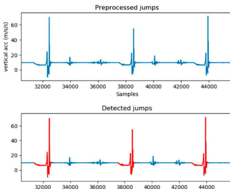
**Figure 9.** The jumping activity recognition algorithm. On top, the vertical acceleration signal of a recording including three consecutive jumps; the bottom figure (in red) depicts the part of the signal that the algorithm has classified as separate jumps.
