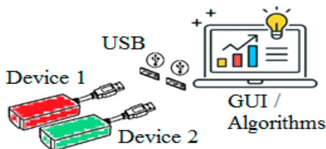
**Figure 2.** Graphical depiction of the system adoption. After data collection for a specific task, the device(s) are plugged-into a computer via USB, where a GUI will use back-end algorithms to process the data gathered in the device(s) and visualize the results to the end-users.
