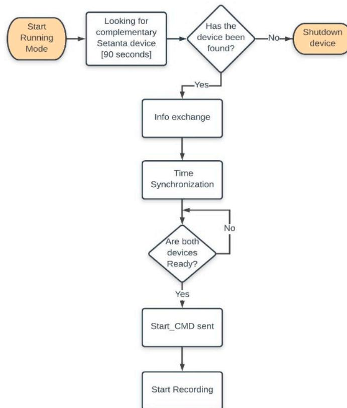
**Figure 5.** “Running” mode flowchart.
