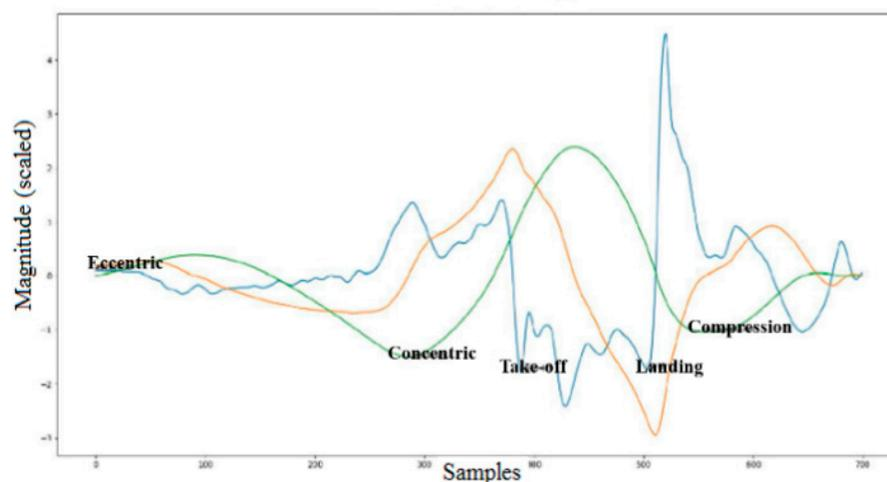
**Figure 10.** Example of event detection from the accelerometer in a countermovement jump. Force (blue), velocity (red), and displacement (green) curves are plotted and manually scaled to be shown in the same graph.
