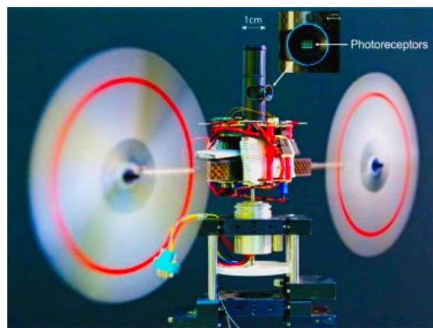
**Figure 24.** VODKA sensor mounted onto an MAV [81].
