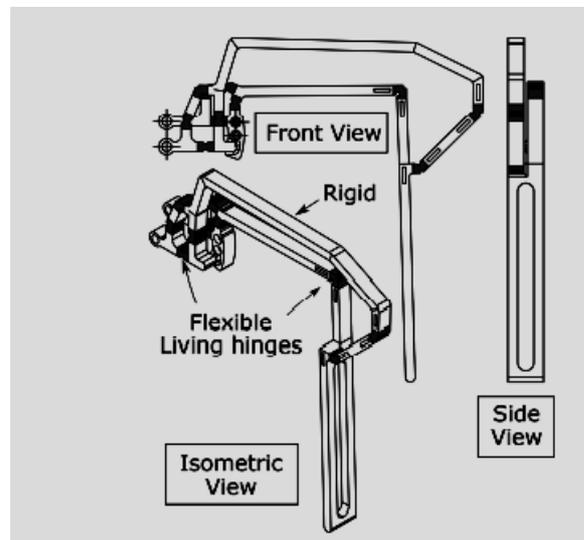
**Figure 22.** Computer-aided design of the arm wing structure mimicking a Bat's wing [75].
