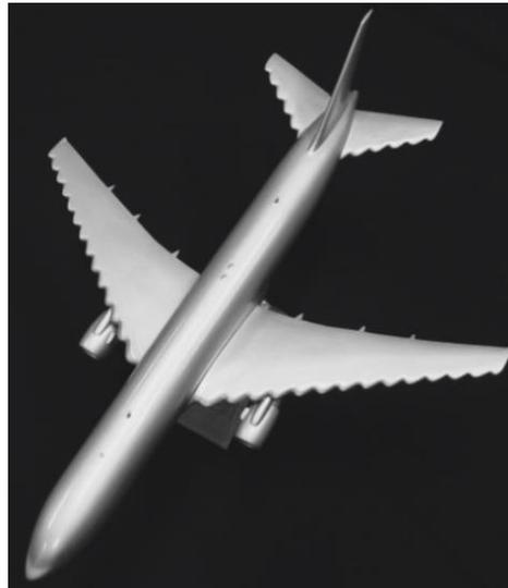
**Figure 16.** Tubercles on the leading edge of the wings and stabilizers of an aircraft [64].
