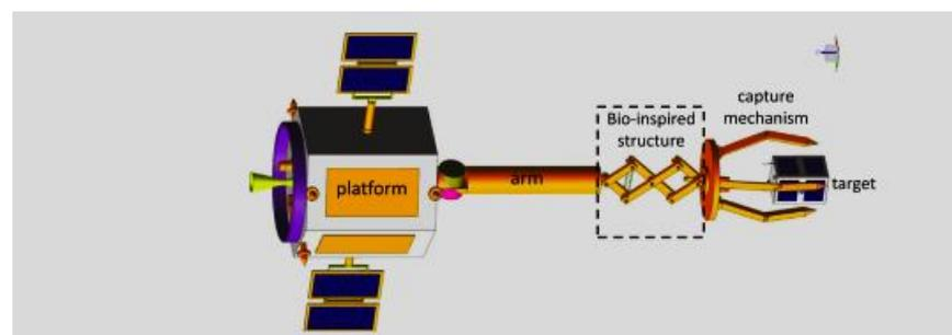
**Figure 25.** An in-orbit capture, with the BIQS system to suppress post-capture vibrations [93].
