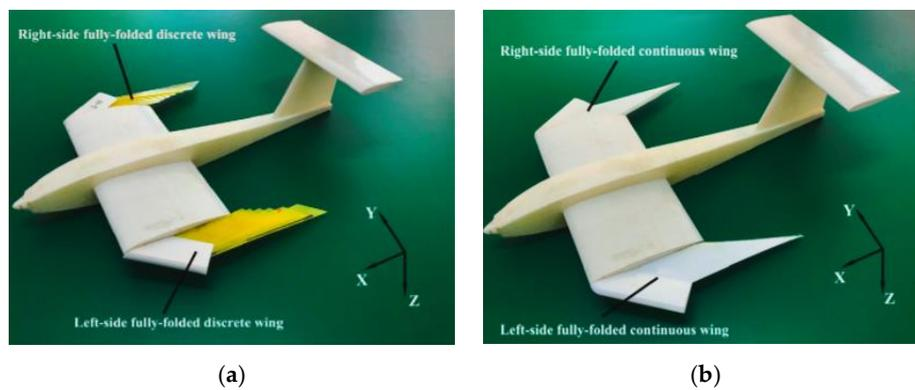
Figure 20. Models fabricated for wind tunnel testing (a) Completely folded, discrete wing design (b) Completely folded, continuous wing design [72].
