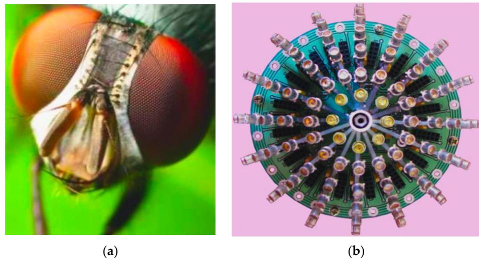
**Figure 23.** Optic sensors based on Elementary Motion Detection (a) Compound eye of a fly (b) A bio-mimicked synthetic compound eye [80].
