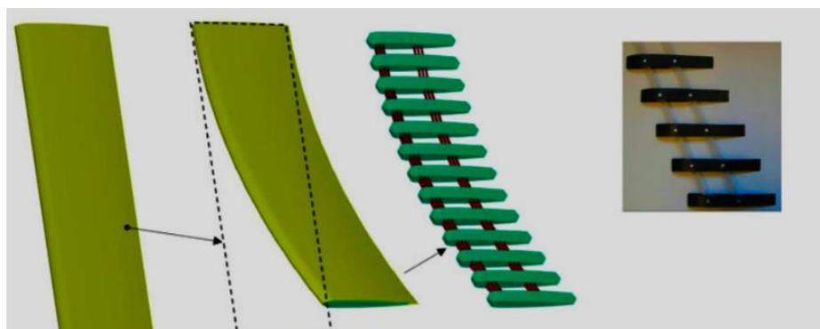
**Figure 17.** Design for a flexing parallelogram wing [66].
