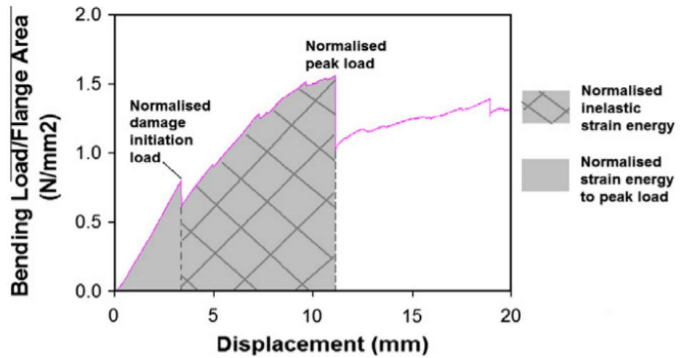
Figure 3. Definition of analysis metrics for T joint performance [25].
