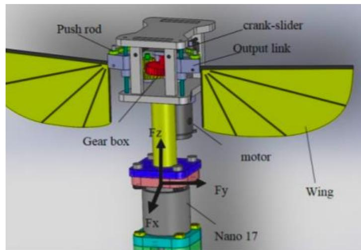
**Figure 18.** Mechanism for flapping to analyse wing deformations [68].
