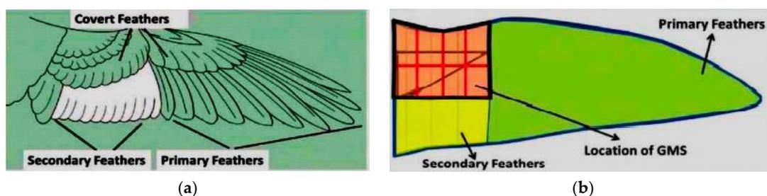
Figure 21. Mechanisms to offset turbulent gusts of wind (a) covert feathers in birds (b) positioning of a GMS unit [74].
