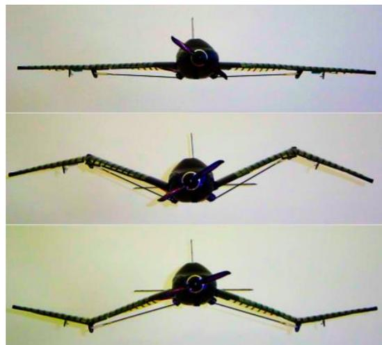
**Figure 15.** Change in wing structure based on variable gull morphing capabilities [62].
