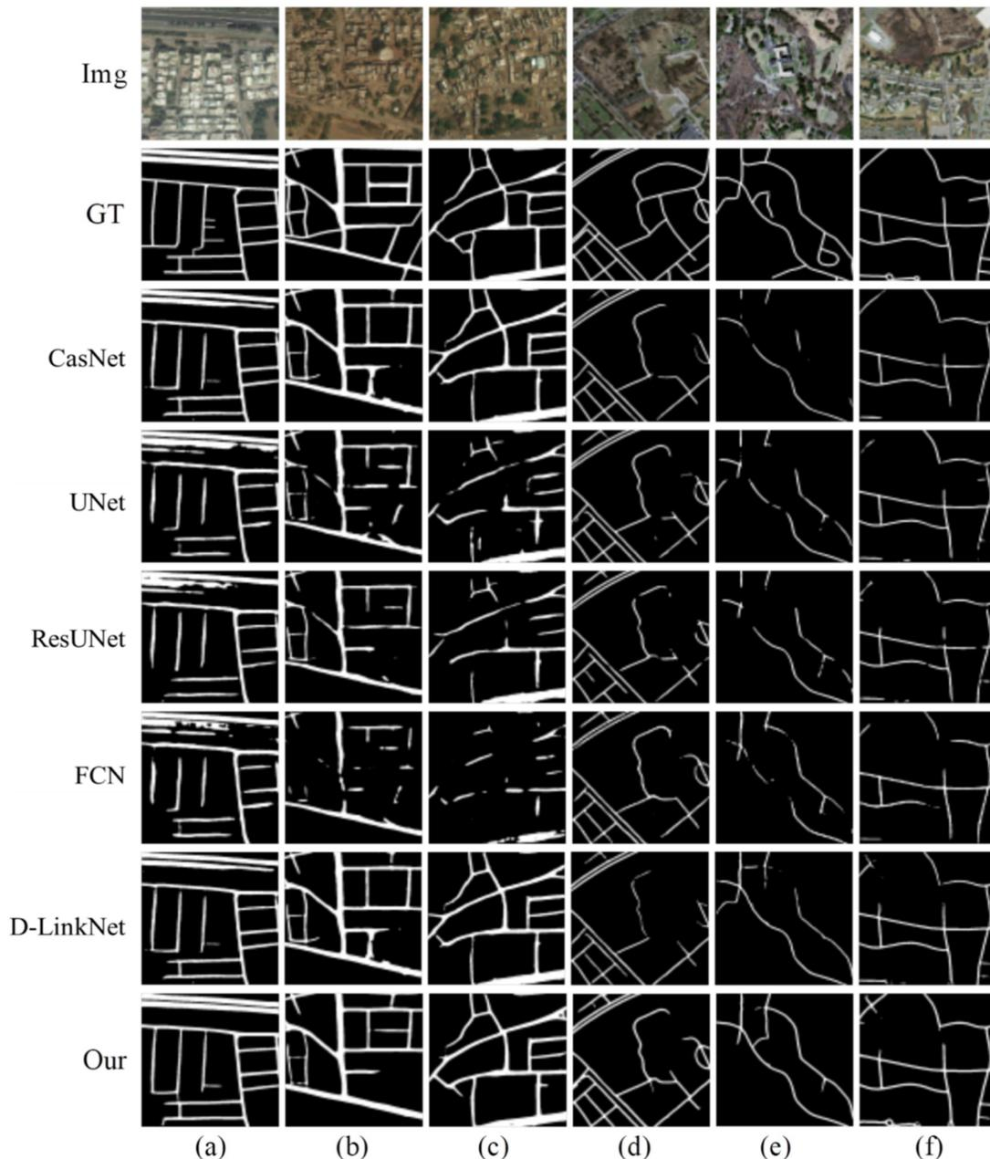
**Figure 4.** Examples of road extraction obtained by the compared methods. (a–c) Selected from the DeepGlobe dataset, and (d–f) showed on the Massachusetts dataset.
