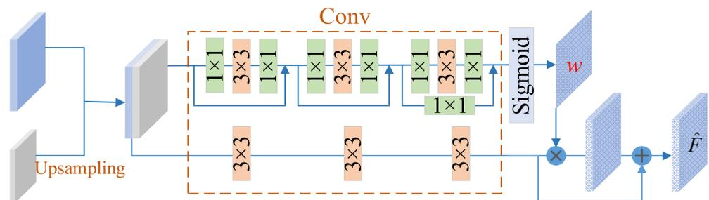
**Figure 2.** Attention mechanism (AM). The features of adjacent layers are first up-sampled to the same size, and are then passed through a series of convolution operations to obtain the attention weight map,  $w$ , and the refined features,  $\hat{F}$ .
