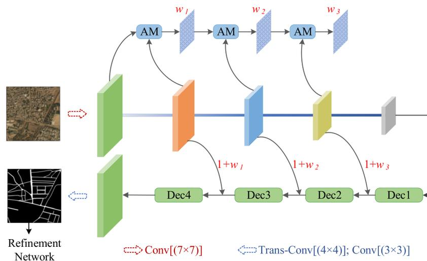
**Figure 1.** The architecture of the proposed network. A self-attention mechanism is exploited to enhance the inter-layer features. The final road maps are obtained through a refinement network.
