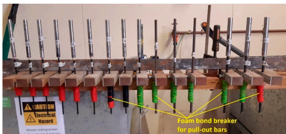
Figure 4. Pull-out bars taped with bond breaker foams before casting.
