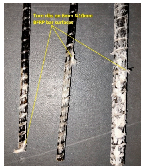
Figure 14. Wear and tear on rib fibres on the pulled-out bar surface.
