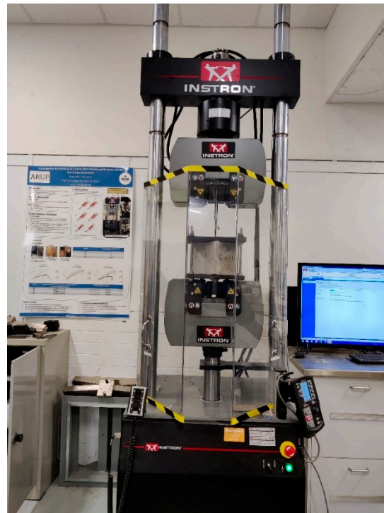
Figure 7. Universal testing machine with automated data acquisition system for pull-out testing.
