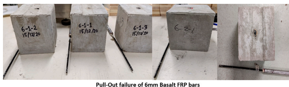
Figure 11. Pull-out failure of 6-mm BFRP bar specimens.
