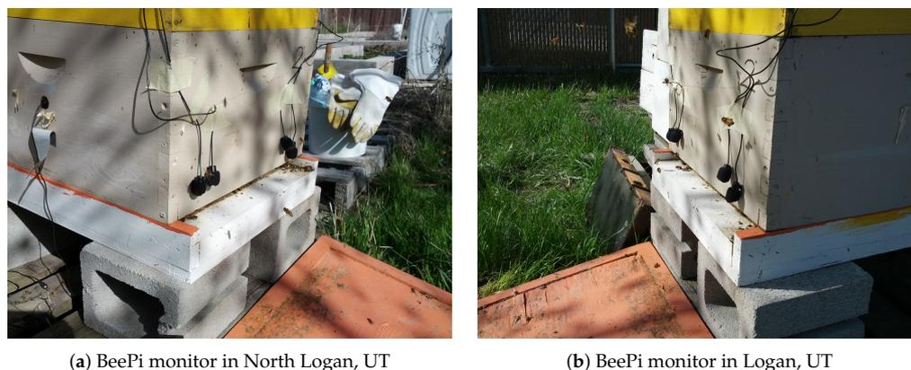
**Figure 2.** Microphones placed  $\approx 10$  cm above landing pads in BeePi monitors in North Logan, UT (a) and Logan, UT (b).
