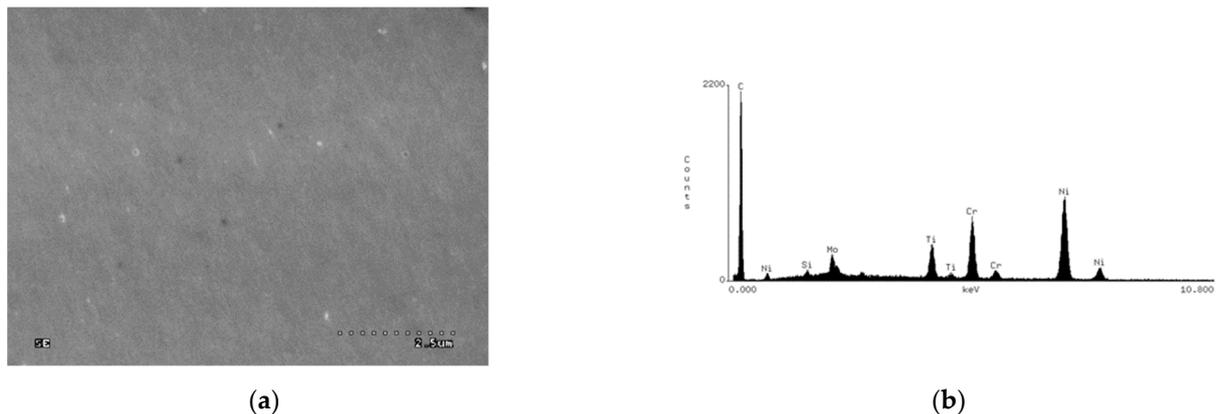
**Figure 1.** Surface of a sample with a carbon coating (a) and an EDS spectrogram from the sample surface (b).
