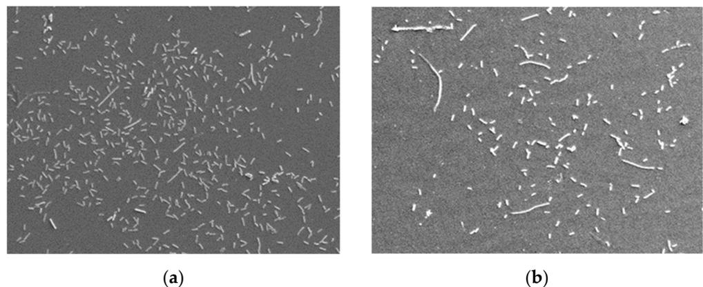
**Figure 7.** Sample surfaces with adhering bacteria (a) Ni-Cr alloy sample without a coating. (b) Ni-Cr alloy sample with a carbon layer.
