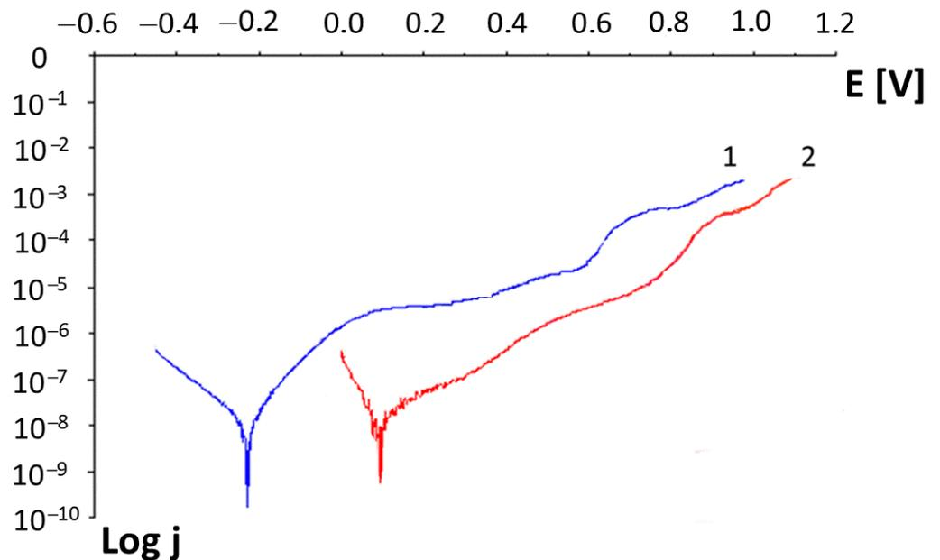
Figure 5. Exemplary current-potential characteristics; 1–Ni-Cr alloy sample with a carbon layer, 2–Ni-Cr alloy sample without a coating.
