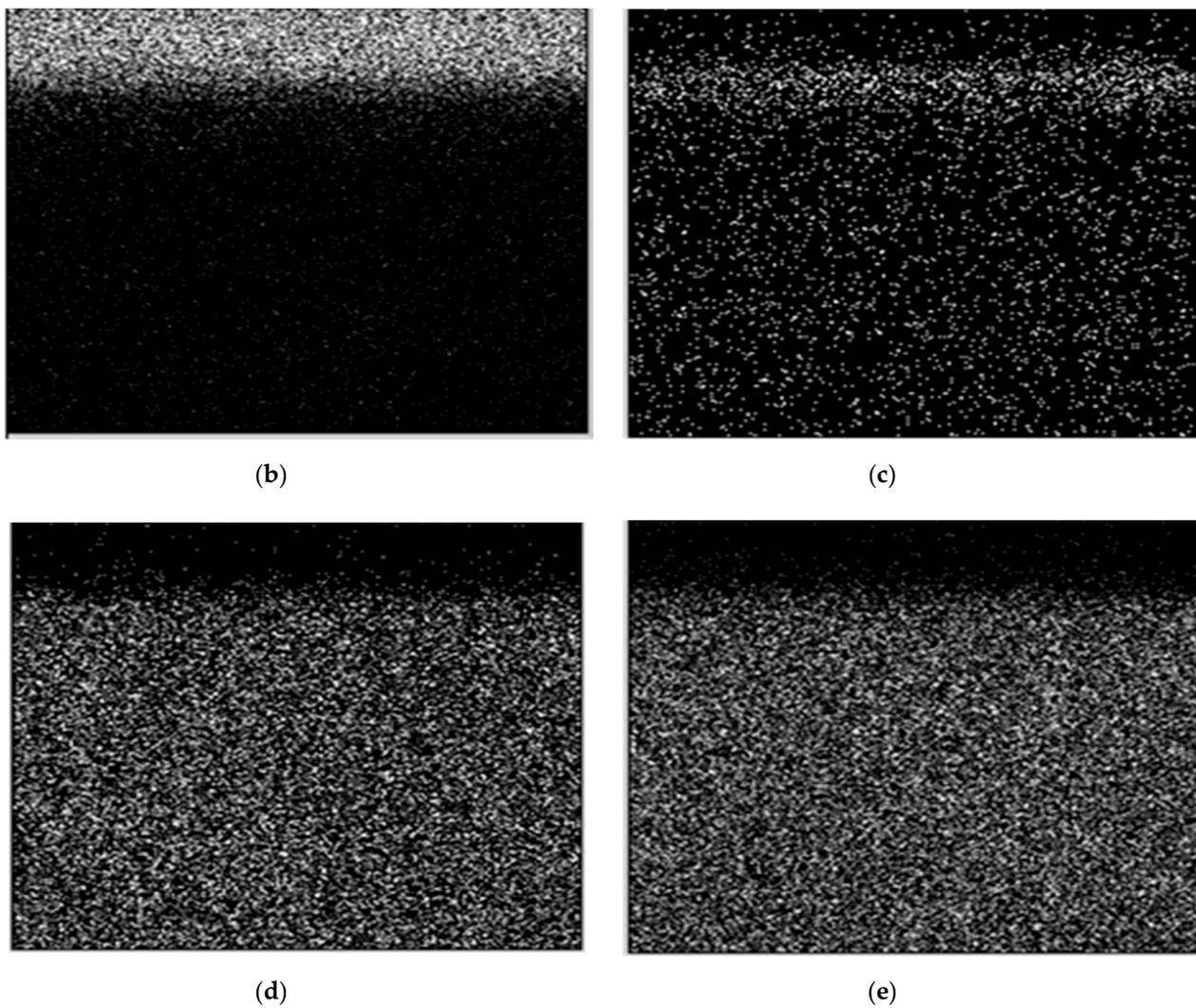
**Figure 2.** Microscopic image of a sample's cross-section with the surface element distributions (a) microscopic image, (b) surface distribution of carbon, (c) surface distribution of titanium, (d) surface distribution of nickel, (e) surface distribution of chromium.
