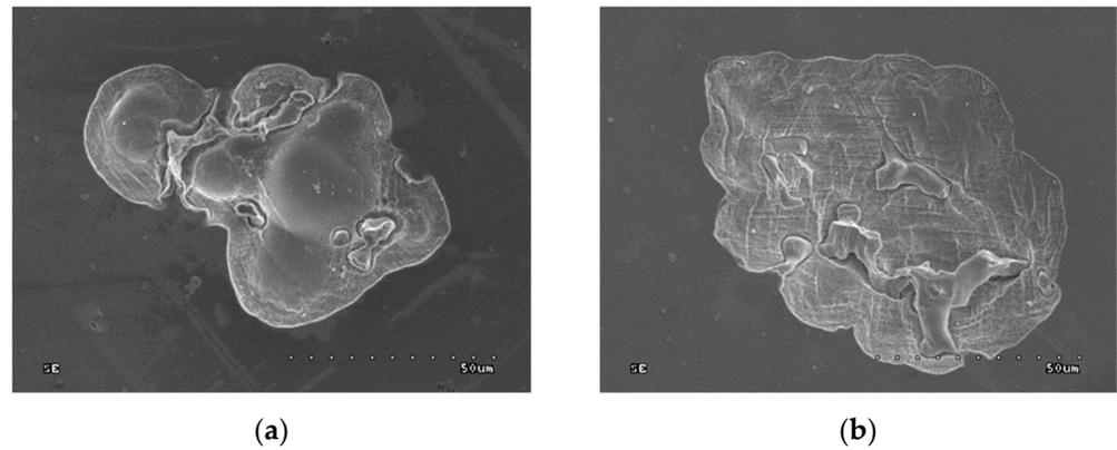
**Figure 6.** Image of the pits after corrosion tests, (a) sample without a coating, (b) sample with a coating.
