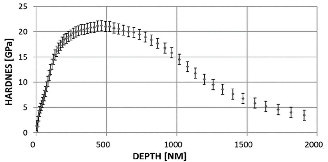
Figure 4. Hardness in the function of the depth of the forced-in penetrator.
