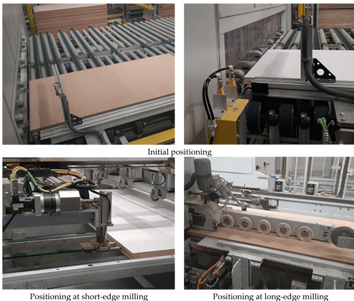
Figure 2. Positioning at edge milling.
