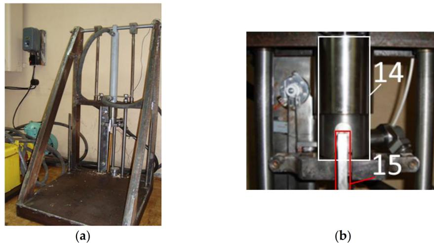
**Figure 4.** General view of the bench (a) and (b) the measuring hydraulic cylinder 14 with the cutter 15, pressure and displacement indicators.
