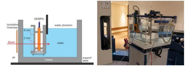
**Figure 8.** Schematic drawing ((**left**), not to scale) and picture (**right**) of the water phantom setup. The beam enters from the left and passes through the reference ionization chamber before entering the water phantom. The GEMPix is inserted in a watertight box, which is mounted on the positioning system of the phantom. Therefore, depth scans are possible by remotely changing the distance between beam entrance window and GEMPix box.
