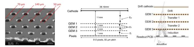
**Figure 2.** (Left) magnified image of a GEM foil. (Centre) scheme of a typical triple GEM in the GEMPix detector and the electric transport fields: drift field (ED), transfer fields (ET) and induction field (EI). (right) electron multiplication (source: CERN).
