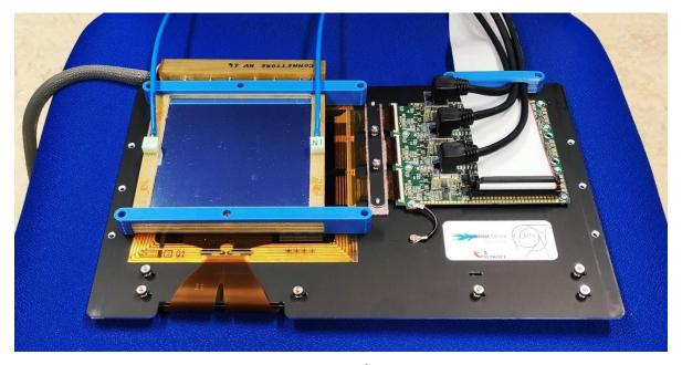
**Figure 16.** The LaGEMPix prototype. The triple GEM  $10 \times 10$  cm<sup>2</sup> stack coupled to the optical readout matrix is on the left side; on top, there is the thin Mylar window. The readout boards and the cables to connect the detector to the FPGA module are on the right side.
