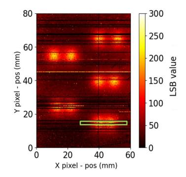
**Figure 17.** Heat map of the Cu mask for 40 kV X-rays. A Region of Interest (ROI, green lines) was set on the holes in 3 mm distance. The spatial resolution was estimated by fitting the profile in the ROIs by a Gaussian function.
