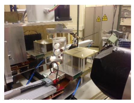
Figure 11. The experimental setup for proton radiography [25].
