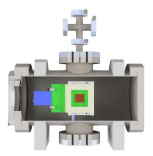
**Figure 18.** A cross-sectional view of the planned vacuum vessel housing the GEMTEQ for sealed and low-pressure applications. The GEMTEQ is located in the centre of the vacuum vessel and the colors show the different materials and components: the aluminum vessel (gray), the FITPix (blue), the PCB (green), the GEM frames (beige) and the Pixelman ASICs (brown). The GEMs are not included in this drawing.
