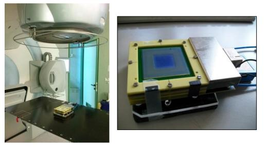
**Figure 6.** The GEMPix placed in position for irradiation with the Elekta Synergy Linac at the Tor Vergata Radiotherapy Centre (**left**) and the EBT gafchromic film placed on the detector window after irradiation (**right**) [21].
