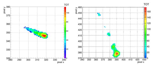
**Figure 15.** Examples of particle tracks measured with the GEMPix: a proton track (from neutron irradiation) with a visible increase in the energy deposition towards the end of the track (**left**) and an electron track (from <sup>137</sup>Cs irradiation, **right**).
