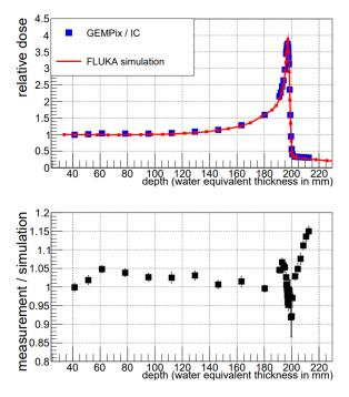
**Figure 9.** The upper plot shows the Bragg curve for 200 mm range in water, measured by the GEMPix and calculated with FLUKA. The lower plot shows the ratio of the experimental data to the FLUKA curve. The data points match the simulation within  $\pm 15\%$ .
