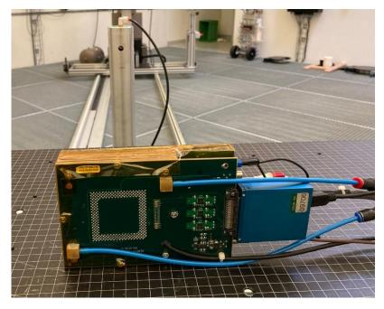
**Figure 13.** The GEMPix detector (foreground) set up for measurements with an AmBe source (the metal cylinder housing the source is visible in the background).
