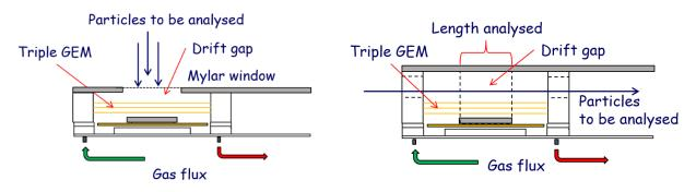
Figure 4. Head-on (left) and side-on (right) configuration of the GEMPix.
