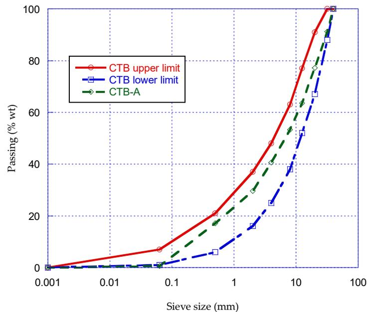
Figure 4. Cement-treated bases A (CTB-A) aggregates skeleton.
