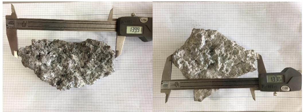
Figure 2. Untreated siderurgical aggregates.
