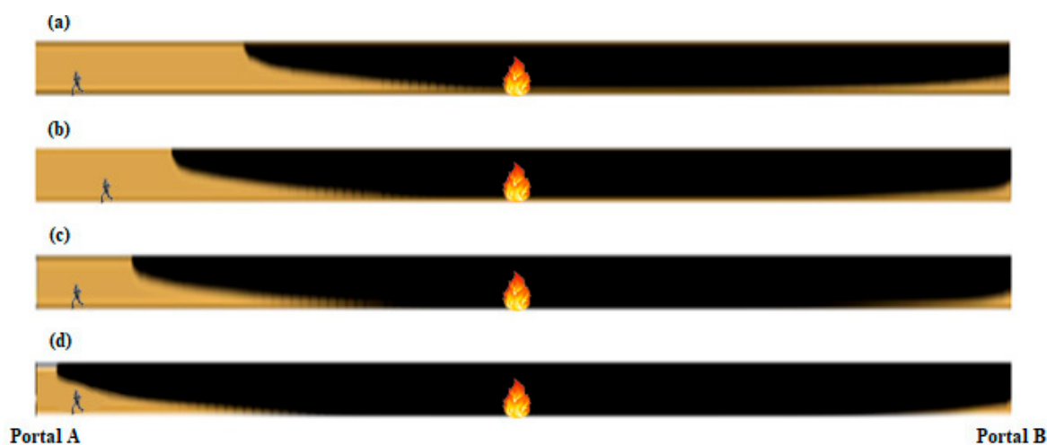
Figure 9. Contours of smoke propagation within the tunnel investigated, after 10 min from the start of fire, when the burning vehicle is in the middle of the tunnel length: (a) 8 MW; (b) 30 MW; (c) 50 MW; (d) 100 MW.
