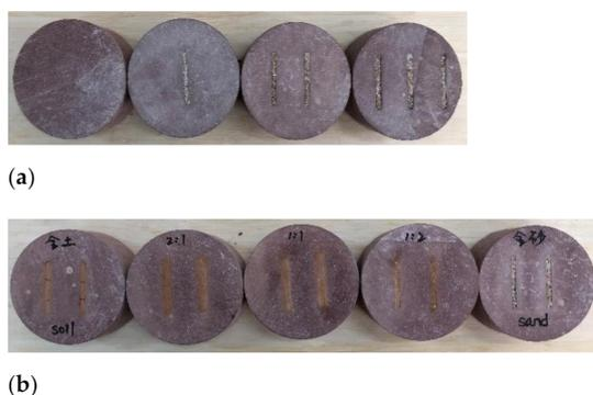
**Figure 4.** (a) Specimens with different numbers of cracks. (b) Specimens with different filling materials.
