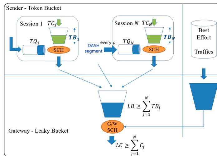
**Figure 2.** Proposal for the transmission structure for an internet protocol (IP)-based terrestrial digital broadcasting system. The token bucket can accommodate burst segment files, and the leaky bucket can be transmitted at a constant bit rate (CBR).
