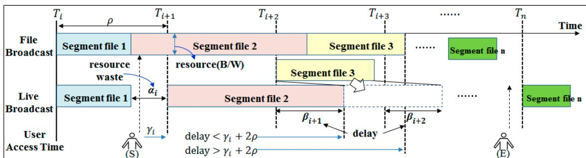
**Figure 1.** Transmission schemes that transmit segment files of variable sizes in a broadcasting network with fixed resources. The file broadcast scheme successively transmits segment files. The live broadcast scheme periodically transmits segment files.
